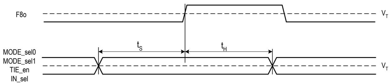
Figure - 15 Input Control Setup and Hold Timing
