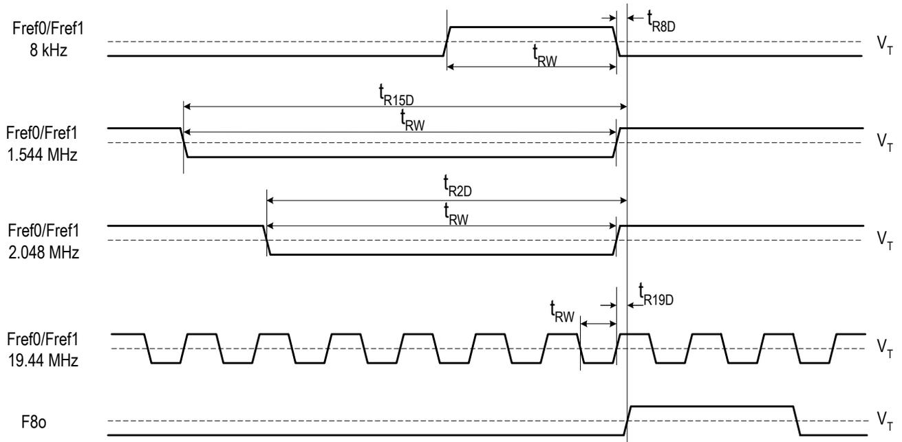
Figure - 12 Input to Output Timing (Normal Mode)
