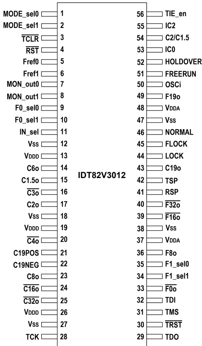
Figure - 1 IDT82V3012 SSOP56 Package Pin Assignment
