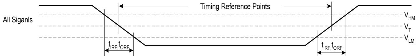
Figure - 11 Timing Parameter Measurement Voltage Levels
