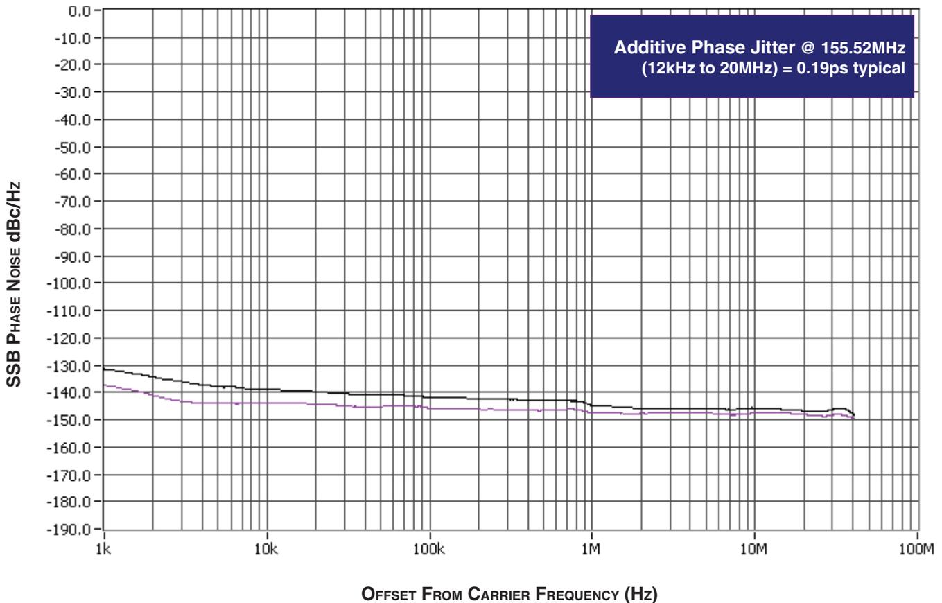
As with most timing specifications, phase noise measurements has issues relating to the limitations of the equipment. Often the noise floor of the equipment is higher than the noise floor of the device.
