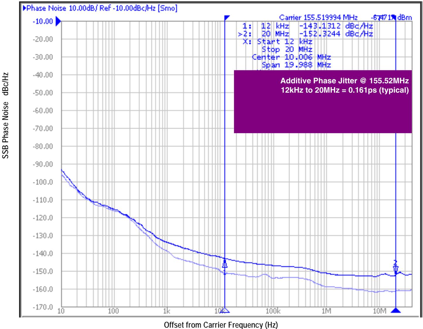
As with most timing specifications, phase noise measurements has issues relating to the limitations of the equipment. Often the noise floor of the equipment is higher than the noise floor of the device. This is illustrated above. The device meets the noise floor of what is shown, but can actually be lower. The phase noise is dependent on the input source and measurement equipment.
