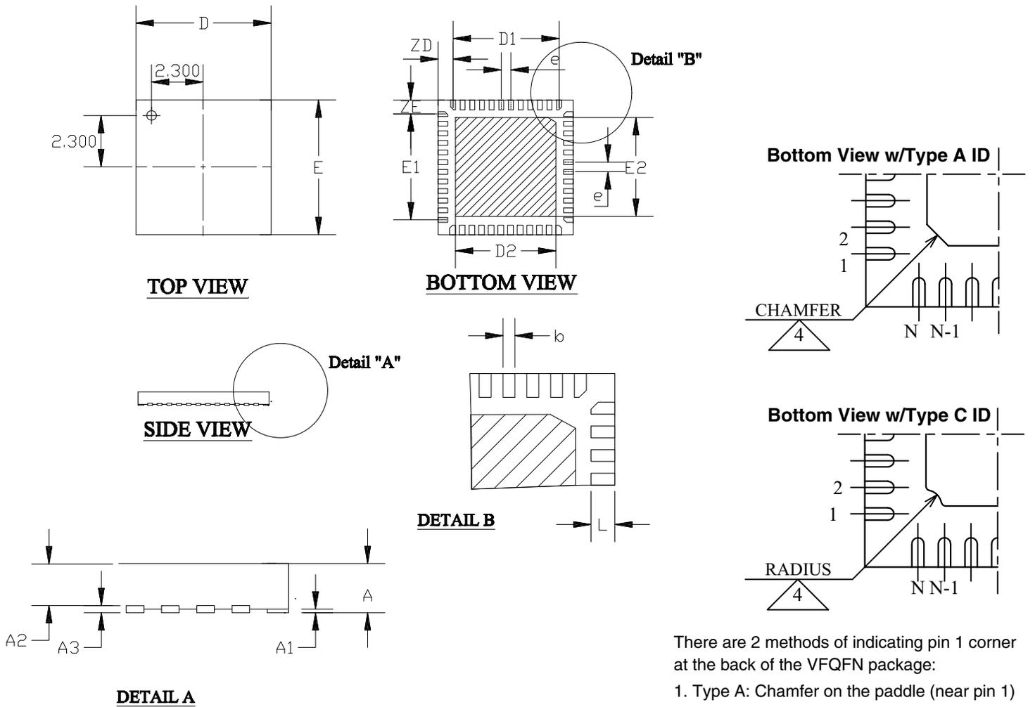
There are 2 methods of indicating pin 1 corner at the back of the VFQFN package:
