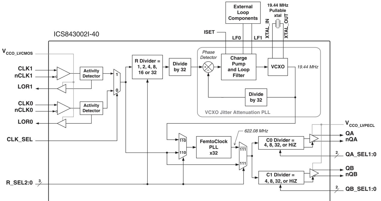
NOTE: 19.44MHz VCXO crystal shown is typical for SONET/SDH device applications.
