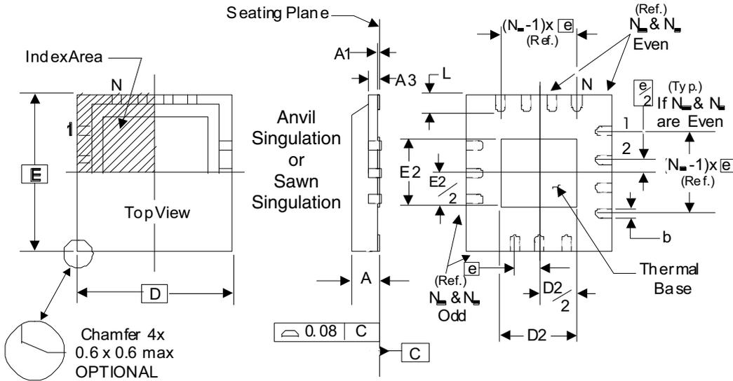
NOTE: The following package mechanical drawing is a generic drawing that applies to any pin count VFQFN package. This drawing is not intended to convey the actual pin count or pin layout of this device. The pin count and pinout are shown on the front page. The package dimensions are in Table 8 below.
