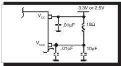
FIGURE 1. POWER SUPPLY FILTERING
