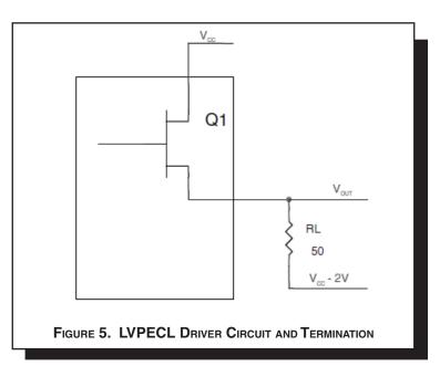
To calculate worst case power dissipation into the load, use the following equations which assume a 50 $\Omega$  load, and a termination
