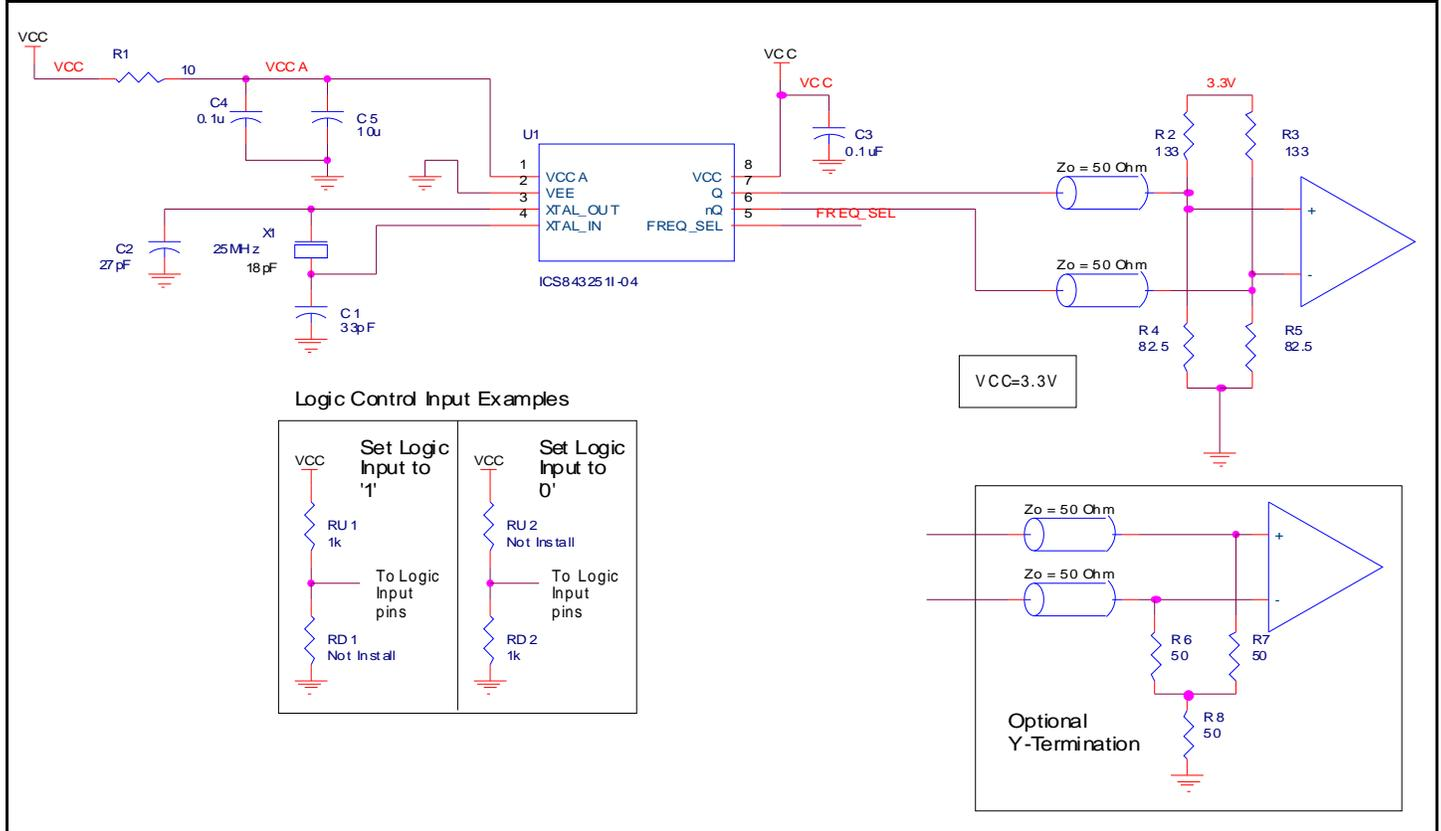
Figure 5. 843251-04 Schematic Example
