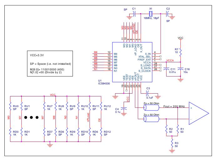
Figure 6A. 84330C Schematic of Recommended Layout
