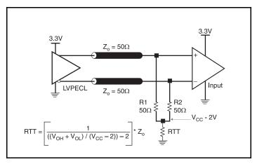
Figure 5A. 3.3V LVPECL Output Termination
