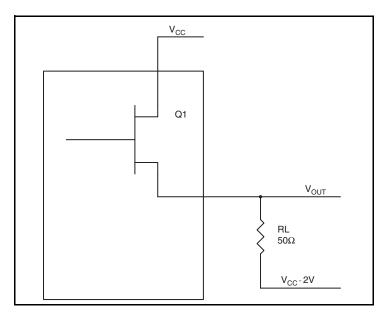
Figure 7. LVPECL Driver Circuit and Termination
