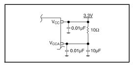
Figure 2. Power Supply Filtering
