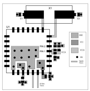
Figure 6B. 84330C PCB Board Layout for 84330C
