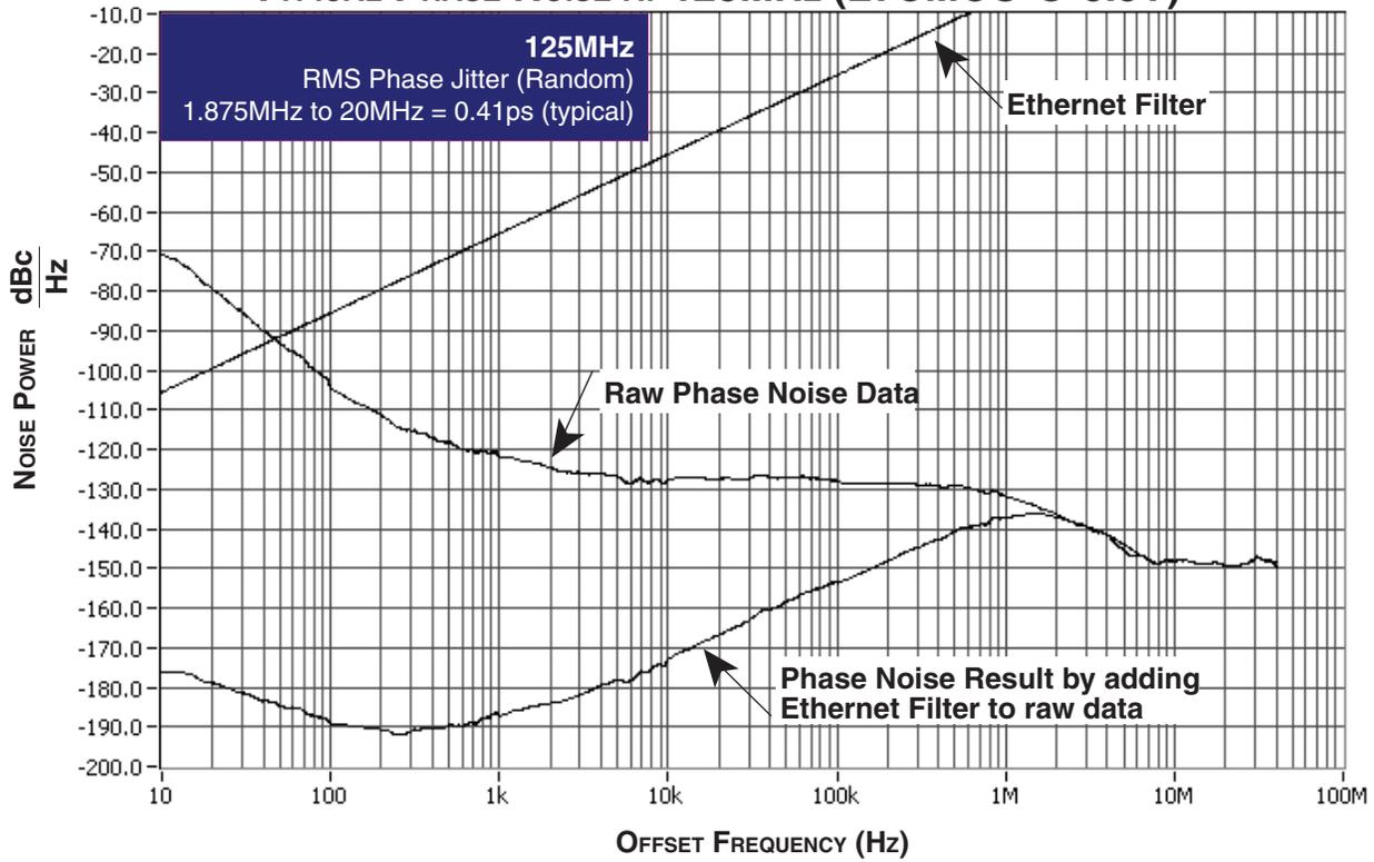
**TYPICAL PHASE NOISE AT 125MHz (LVDS @ 3.3V)**
