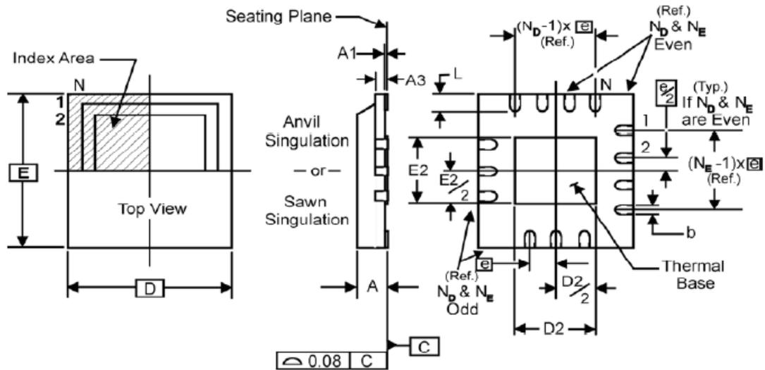
NOTE: The following package mechanical drawing is a generic drawing that applies to any pin count VFQFN package. This drawing is not intended to convey the actual pin count or pin layout of this device. The pin count and pinout are shown on the front page.
