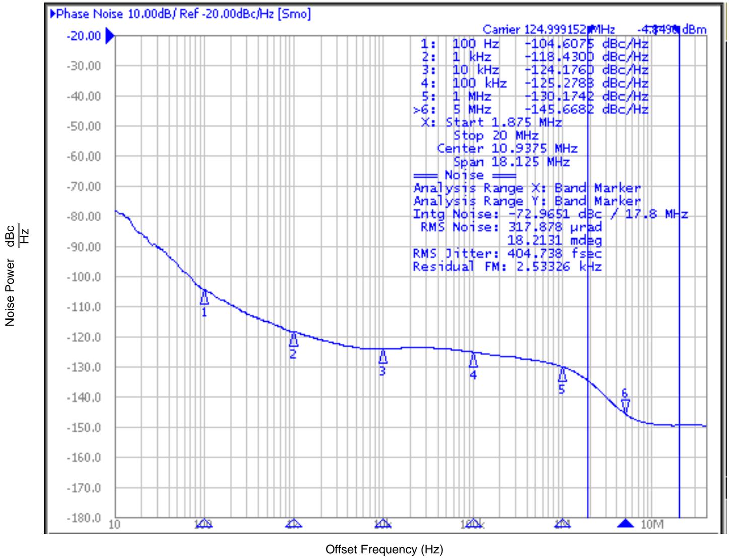
Typical Phase Noise at 156.25MHz (3.3V)
