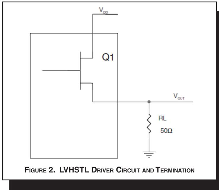
FIGURE 2. LVHSTL DRIVER CIRCUIT AND TERMINATION
