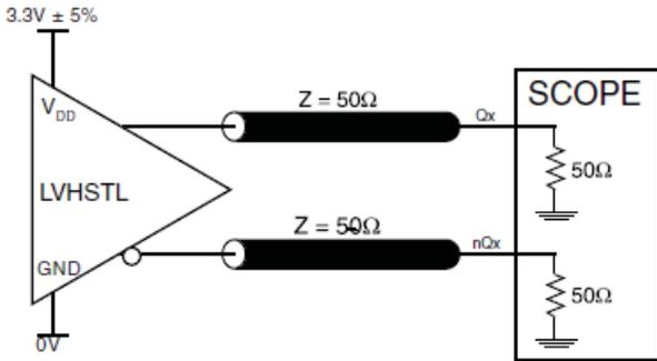
3.3V CORE/3.3V OUTPUT LOAD AC TEST CIRCUIT
