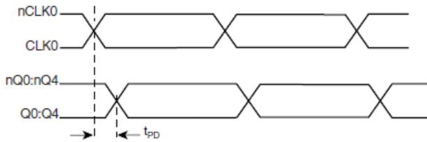
PROPAGATION DELAY (DIFFERENTIAL INPUT)
