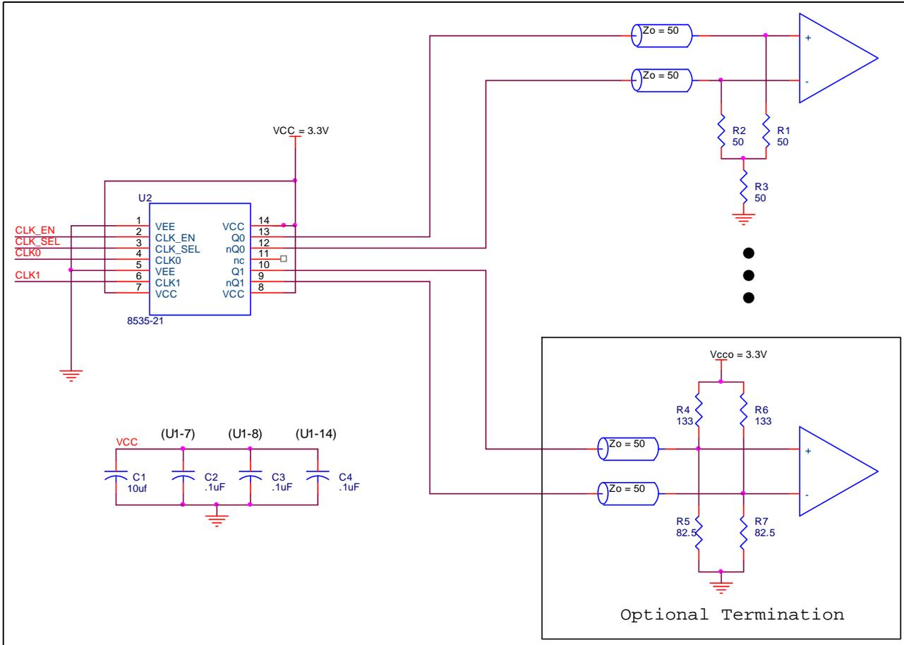
Figure 3. 8535-21 LVPECL Buffer Schematic Example
