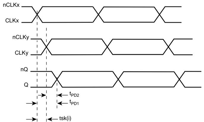
$$tsk(i) = |t_{PD1} - t_{PD2}|$$
