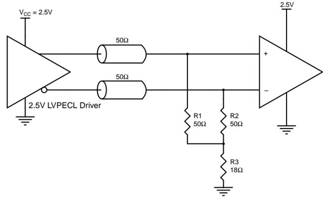
Figure 5C. 2.5V LVPECL Driver Termination Example
