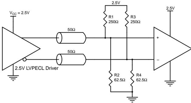
Figure 5B. 2.5V LVPECL Driver Termination Example
