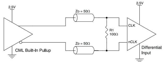
**Figure 3E. CLK/nCLK Input Driven by an IDT Open Collector CML Driver**
