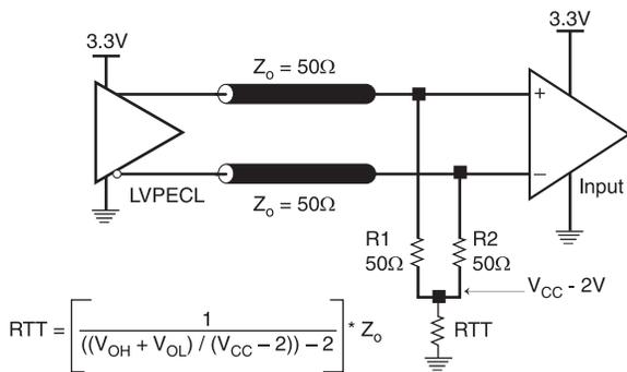
Figure 4B. 3.3V LVPECL Output Termination
