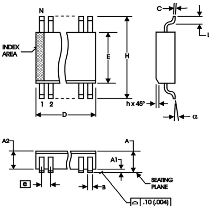
**Table 9A. Package Dimensions for 20 Lead SOIC**
