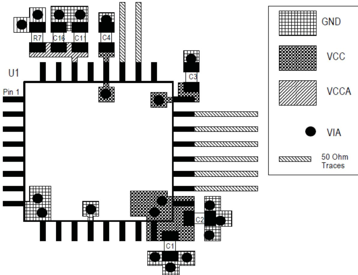
FIGURE 5B. PCB BOARD LAYOUT FOR 879931
