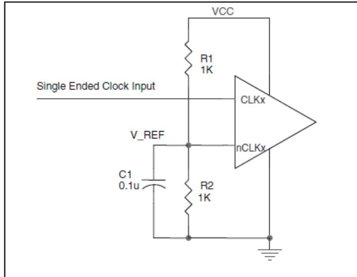
**FIGURE 3. SINGLE ENDED SIGNAL DRIVING DIFFERENTIAL INPUT**
