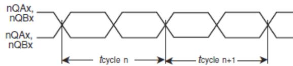
$$t_{jit(cc)} = t_{cycle n} - t_{cycle n+1}$$
