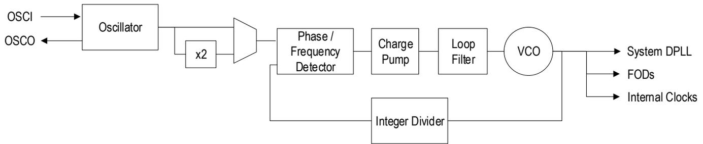
During a device reset, the System APLL is configured by loading the appropriate control register fields from the internal One-Time Programmable memory or an external serial EEPROM, whichever is enabled and has valid contents. After the reset sequence has completed, the System APLL can be re-configured manually over the serial port at any time.
