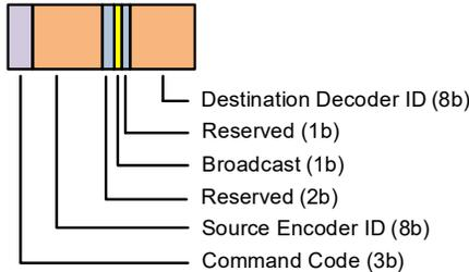
The 8A34011 encoders and decoders supports four Command Codes natively in hardware: PWM\_PPS (000b), PWM\_SYNC (011b), PWM\_READ (010b), and PWM\_WRITE (1000b).
