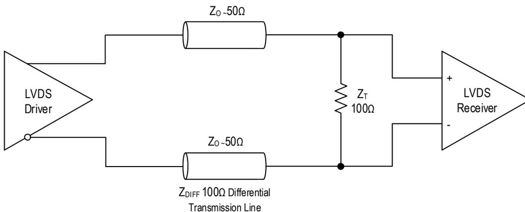
**Figure 50. AC Coupled LVDS Termination**
