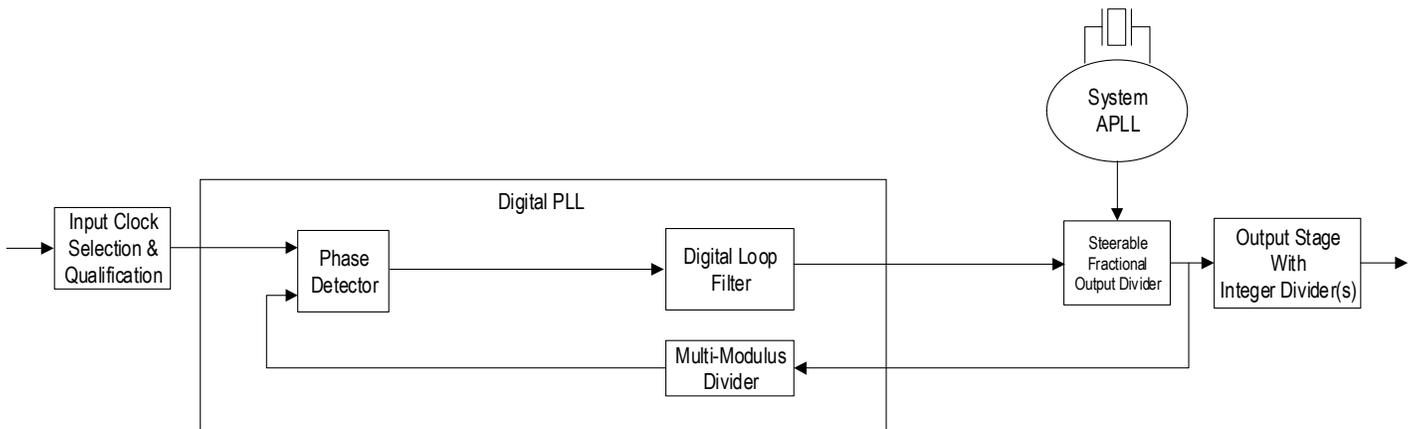
The high-frequency output signal from the System APLL is divided-down by the FOD block to a frequency from 500MHz to 1GHz. The output frequency is unrelated to the System APLL frequency since fractional division is used (for information, see [System APLL](#)). That signal is in turn fed to the output stage, where it is further divided by the integer divider(s) and provided to the output in the selected output format. For more information, see [FOD Multiplexing and Output Stages](#).
