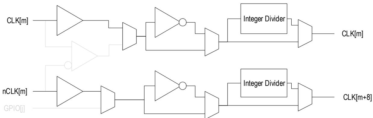
When programmed as differential plus one single-ended as shown in [Figure 7](#), two independent inputs are provided to the 8A34011. This mode can only be used with the GPIOs and input stages shown in the following table. See the INPUT\_0.IN\_MODE bit field.
