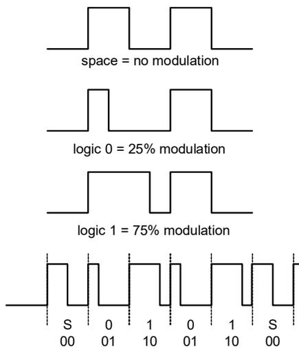
Each input on the 8A34011 can decode information from a carrier clock using pulse-width modulation (PWM). The carrier clock and/or decoded information can then be sent to any DPLL or to the System DPLL.
