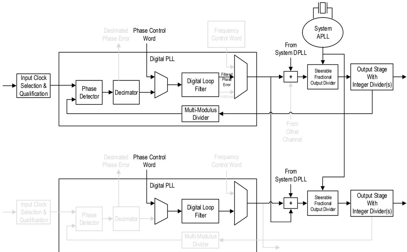
In this example, the IEEE 1588 timestamps are used to calculate the phase offset between the IEEE 1588 master's 1PPS pulse and the IEEE 1588 slave's 1PPS pulse and then align the two pulses by moving the slave's 1PPS pulse in phase. The slave must be able to move the 1PPS pulse by  $\pm 0.5s$ , and the 8A34011 provides this capability.
