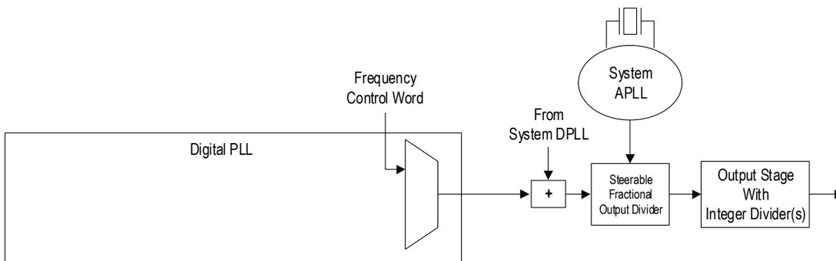
The FCW is a 42-bit 2's-complement value. The FCW has a granularity of  $1.11 \times 10^{-10}$  ppm and a full range of +244.20ppm to -244.08ppm of the nominal DCO frequency. A positive value will increase the output frequency and a negative one will decrease the output frequency. The formula for calculation of the FCW from the fractional frequency offset (FFO) is:
