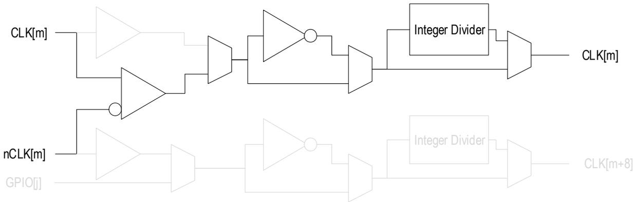
The 8A34011 supports input frequencies up to 1GHz for differential inputs. If the input reference clock frequency is higher than 150MHz, then it must be divided down to the internal frequency (less than or equal to 150MHz) used by the DPLL. An integer divider with a range between 2 to 65536 is provided to divide the signal down to less than or equal to 150MHz. For input reference clock frequencies less than 150MHz, the internal divider can be bypassed. See the INPUT\_0.IN\_MODE bit field.
