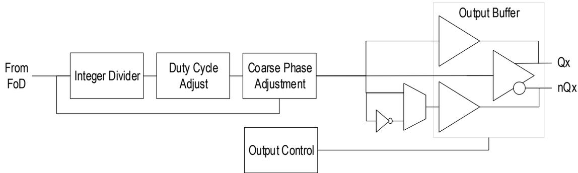
Other than having two copies of each functional block fed from the same FOD, both single and dual output stages behave the same. Similarly, the two paths within the dual output stages behave the same as each other. Descriptions of each functional block are provided in the following sub-sections.
