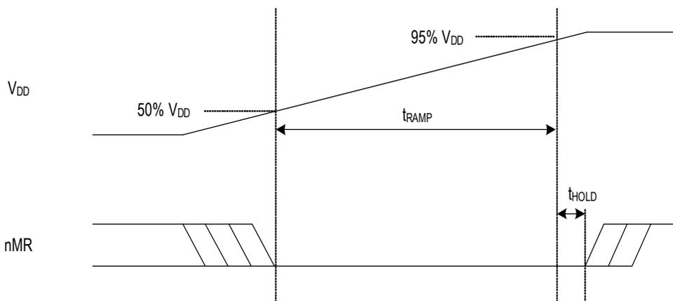
In cases where the device is not powering up and just being reset, a low pulse on nMR of 20ns will be sufficient to reset the device.
