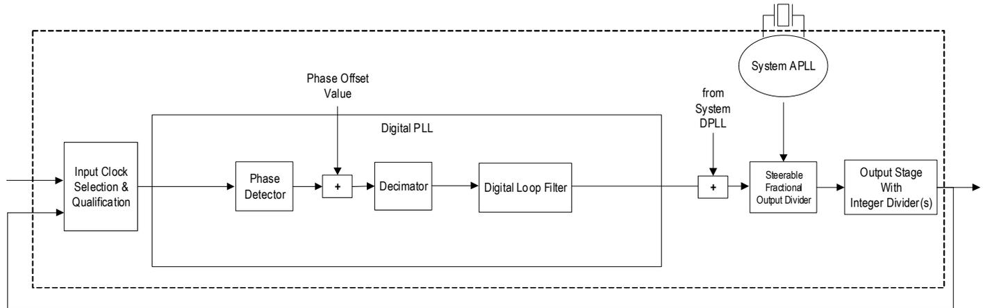
For both ZDPLL and ZDB, the frequency of the external feedback clock must be the same as the reference clock input. For this reason, all of the reference clock inputs must be the same frequency when using automatic reference switching. Otherwise, the external feedback clock must be reconfigured to match the new input reference clock frequency prior to manually switching to the new reference. See the DPLL\_0.DPLL\_CTRL\_2 and INPUT\_0.IN\_MODE bit fields.
