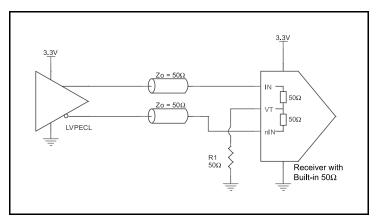
Figure 4B. IN/nIN Input with Built-In 50Ω Driven by an LVPECL Driver
