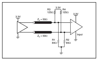
Figure 7B. 3.3V LVPECL Output Termination
