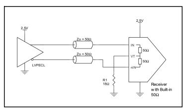
Figure 5B. IN/nIN Input with Built-In 50 $\Omega$  Driven by an LVPECL Driver
