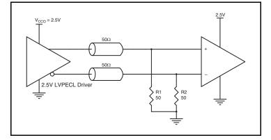
Figure 8C. 2.5V LVPECL Driver Termination Example
