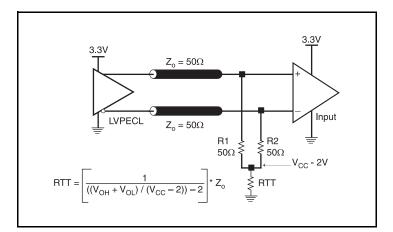
Figure 7A. 3.3V LVPECL Output Termination
