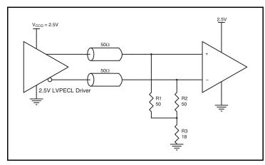
Figure 8B. 2.5V LVPECL Driver Termination Example
