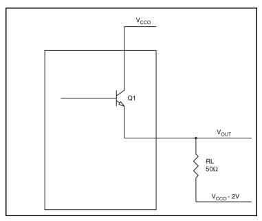
Figure 9. LVPECL Driver Circuit and Termination
