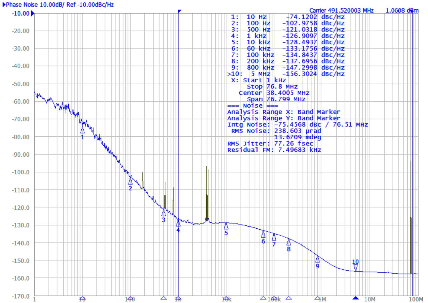
**Figure 12. 245.76MHz Output Phase Noise**
