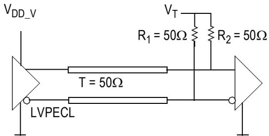
$V_T = V_{DD\_V} - 1.50V$  (250mV Amplitude)
