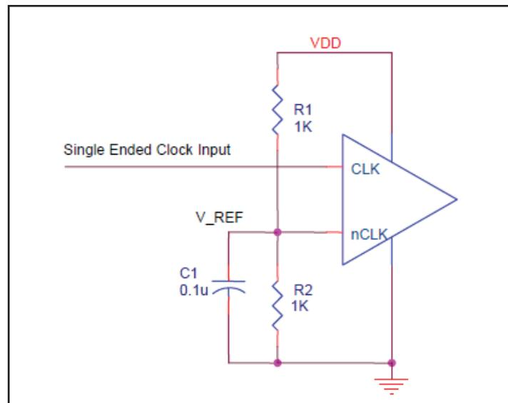
FIGURE 2. SINGLE ENDED SIGNAL DRIVING DIFFERENTIAL INPUT
