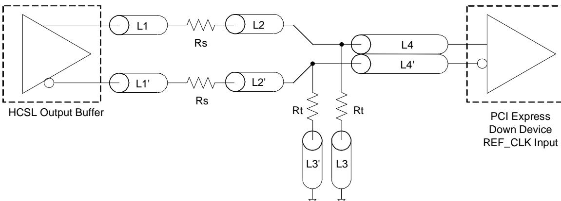
Figure 2: PCI Express Connector Routing
