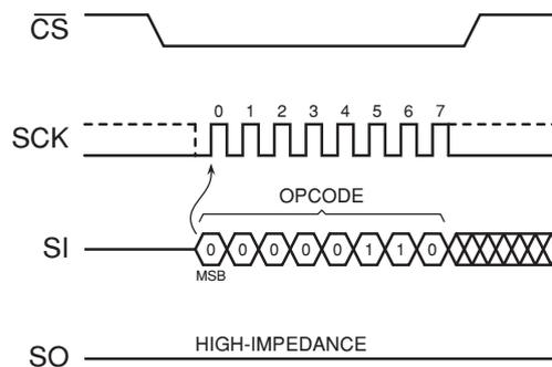
Figure 14. Write Enable
