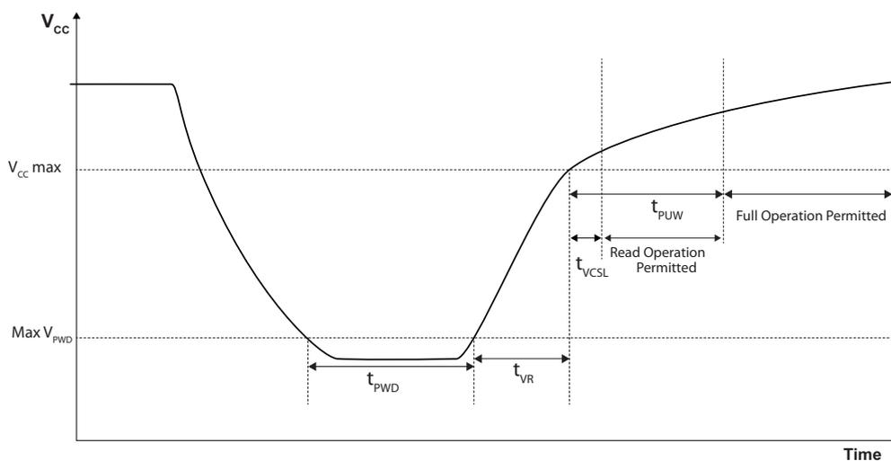
Figure 30. Power-Up Timing
