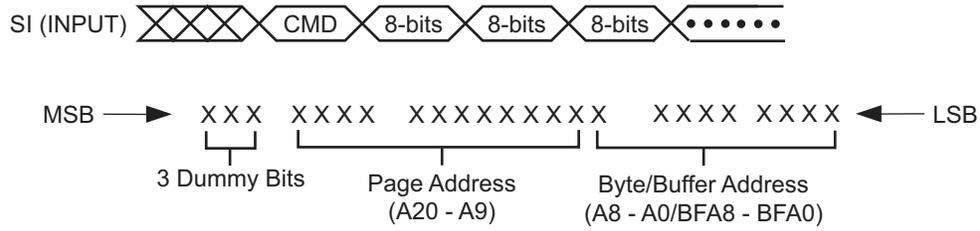
**Figure 21-3. Command Sequence for Read/Write Operations for Page Size 528 bytes**
