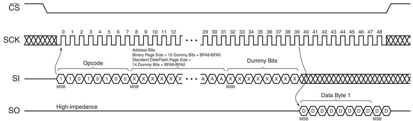
**Figure 25-6. Buffer Read – Low Frequency (Opcode D1h or D3h)**
