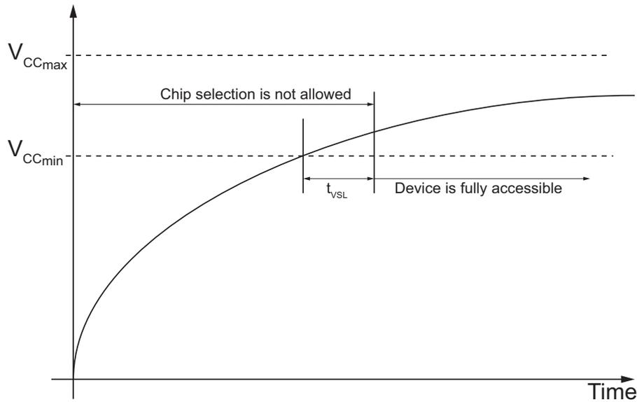
Figure 42. Power-Up Timing and Voltage Levels
