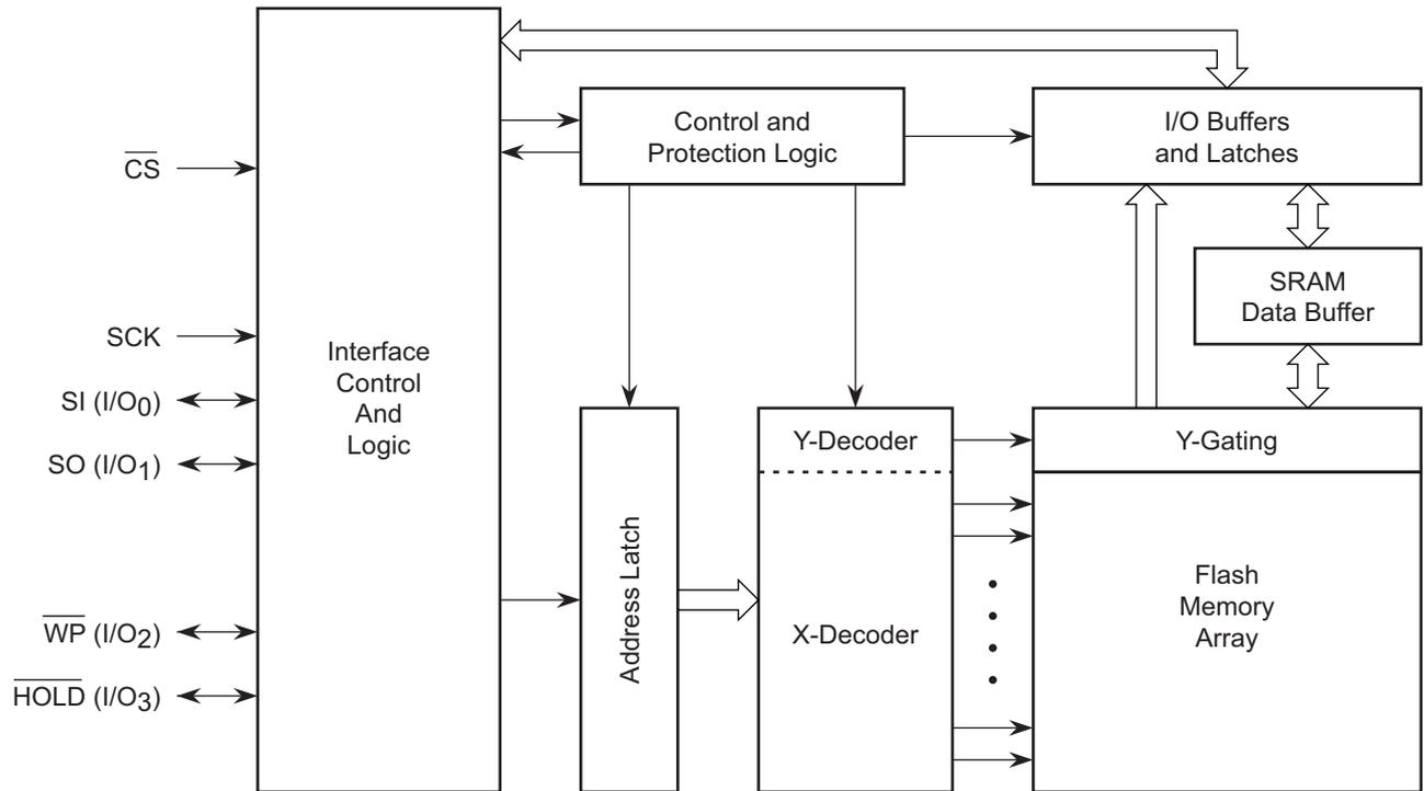
Note: I/O<sub>3-0</sub> pin naming convention is used for Dual-I/O and Quad-I/O commands.
