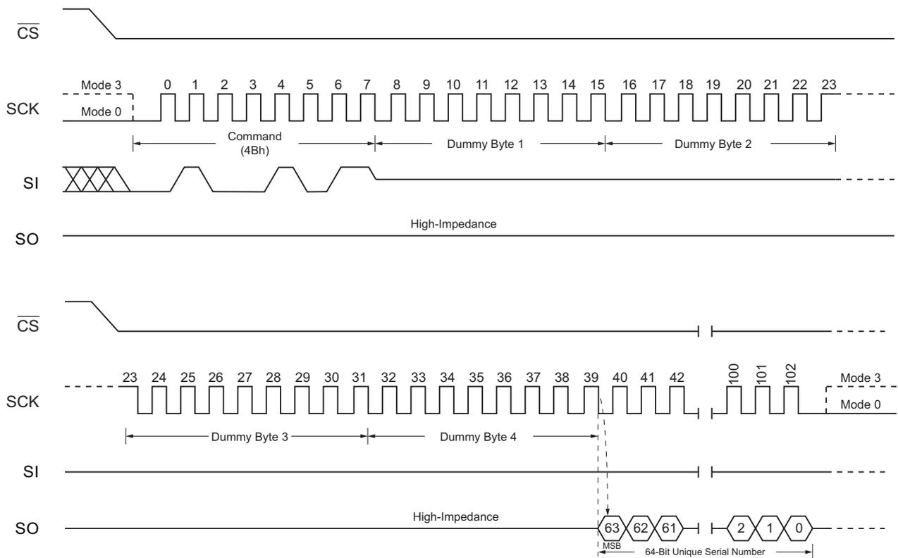
Figure 27. Read Unique ID Timing (SPI Mode)
