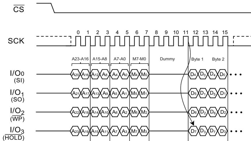
Figure 12. Quad-I/O Read Array with Continuous Read Mode (Previous Command Set M5-4 =1,0)
