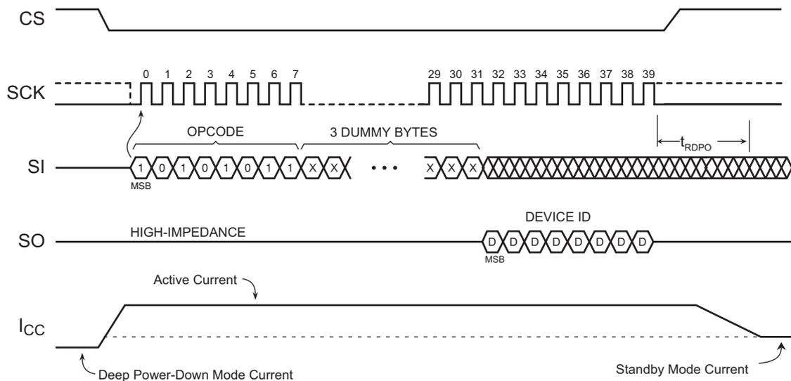
Figure 41. Resume from Deep Power-Down and Read Device ID
