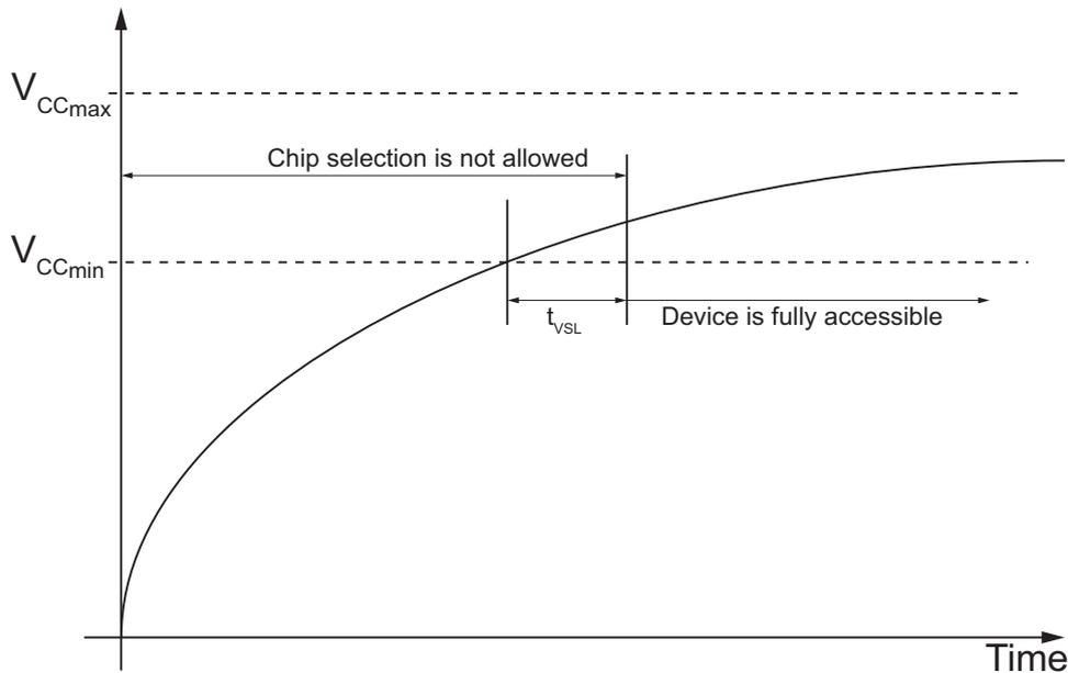
Figure 42. Power-Up Timing and Voltage
