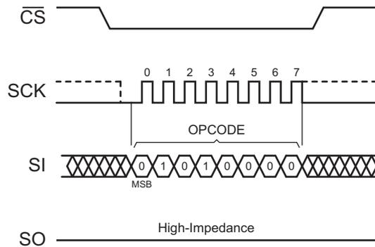
Figure 34. Write Enable for Volatile Status Register
