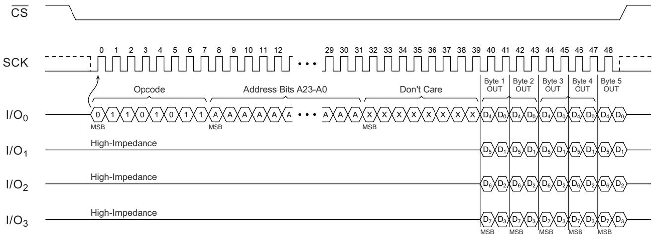
Figure 10. Quad-Output Fast Read Array
