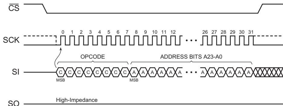
Figure 20. Block Erase Timing
