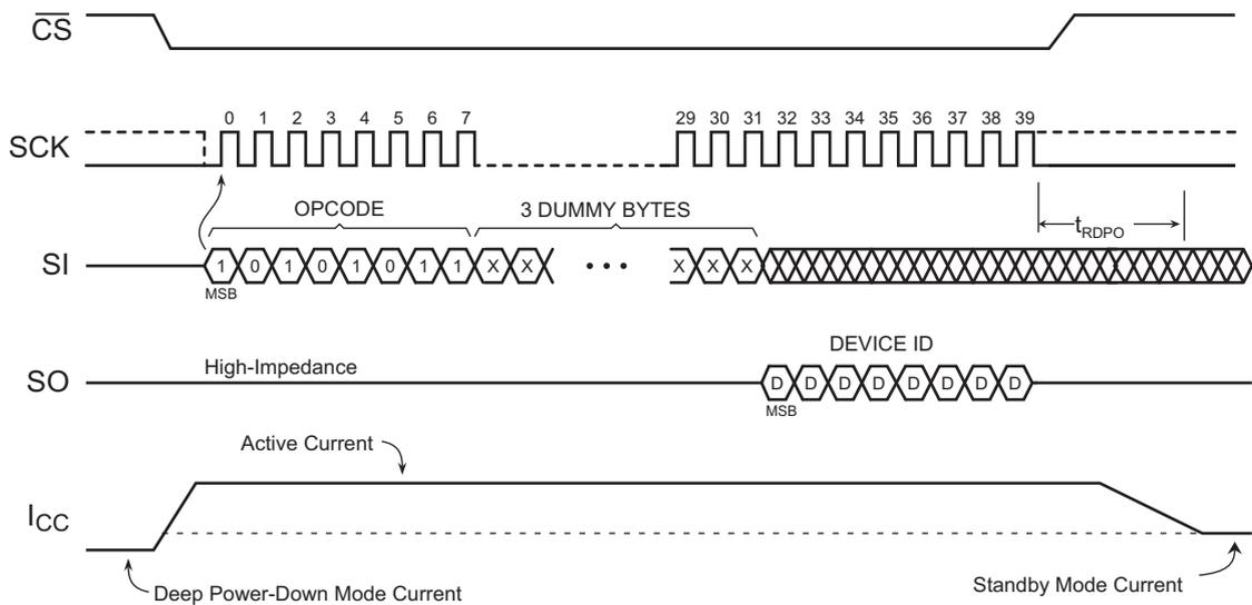
Figure 41. Resume from Deep Power-Down and Read Device ID Timing
