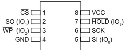
Figure 1. 8-SOIC (0.150" and 0.208") — Top View
