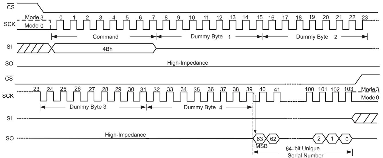
Figure 27. Read Unique ID Timing (SPI Mode)
