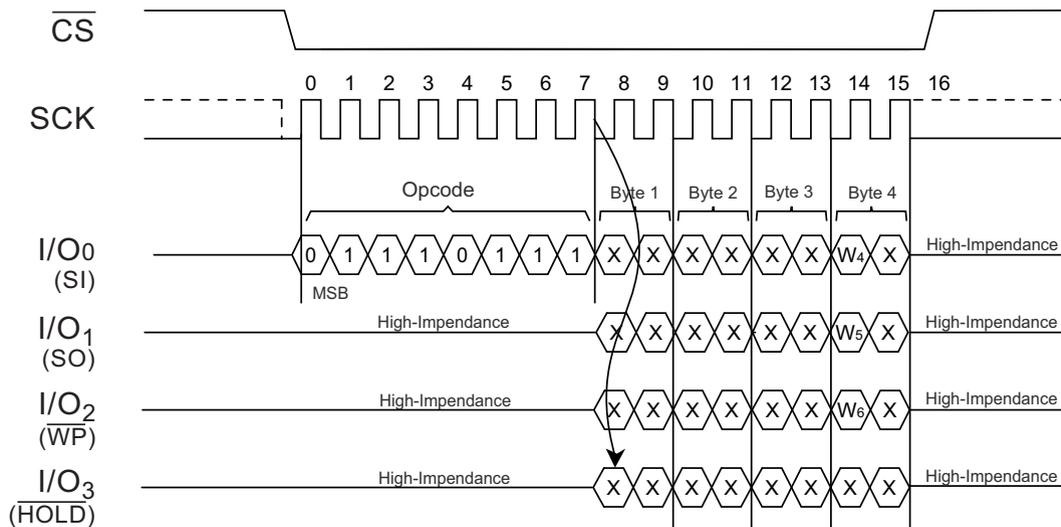
Figure 13. Set Burst with Wrap Timing (SPI Mode)
