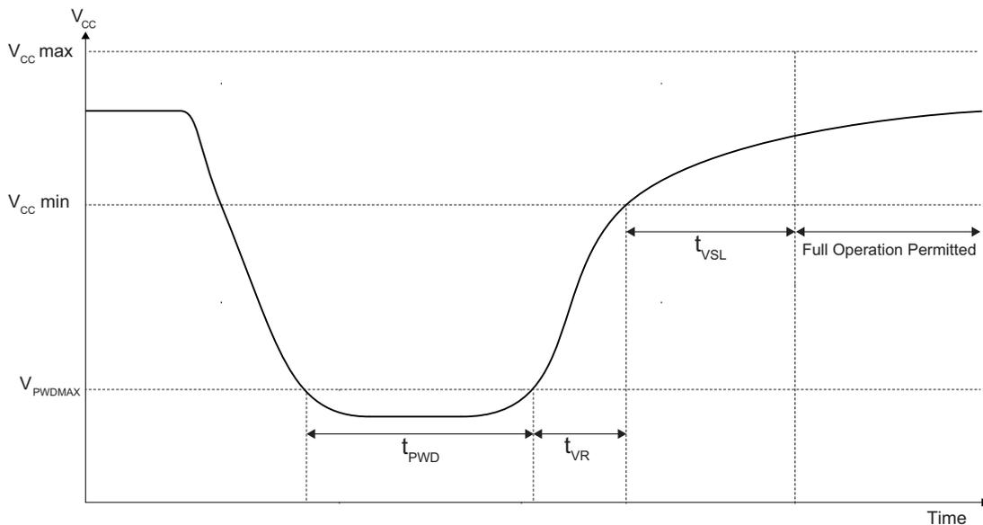
Figure 72. Power-up Timing After Brown-Out
