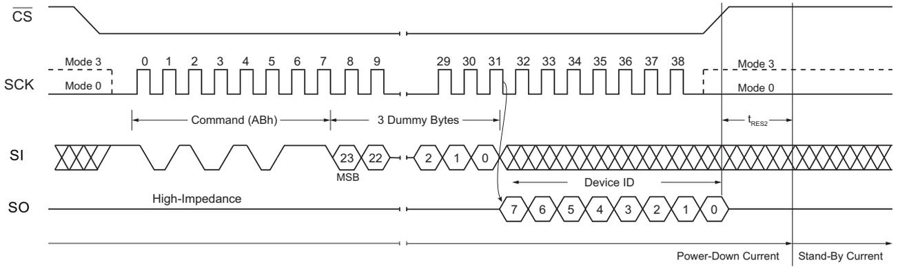
Figure 48. Release Power-Down / Device ID Command (SPI Mode)
