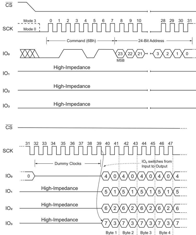
Figure 25. Fast Read Quad Output Command (SPI Mode)
