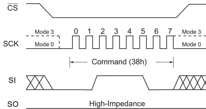
Figure 17. Enable QPI Command (SPI Mode only)
