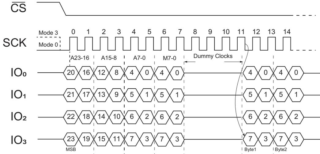
Figure 31. Fast Read Quad I/O Command (Initial command or previous M5-4 = 1,0; QPI mode)
