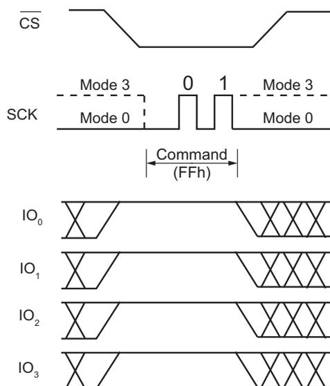
Figure 18. Disable QPI Command for QPI Mode
