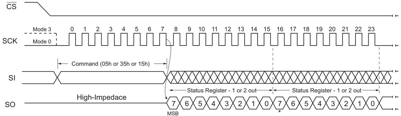
Figure 11. Read Status Register Command (SPI Mode)
