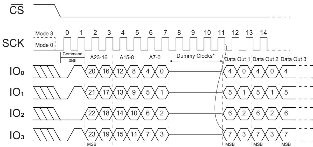
\* = “Set Read Parameters” command (C0h) can set the number of dummy clocks
