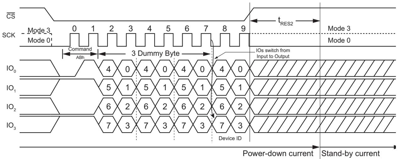
Figure 49. Release Power-Down / Device ID Command (QPI Mode)
