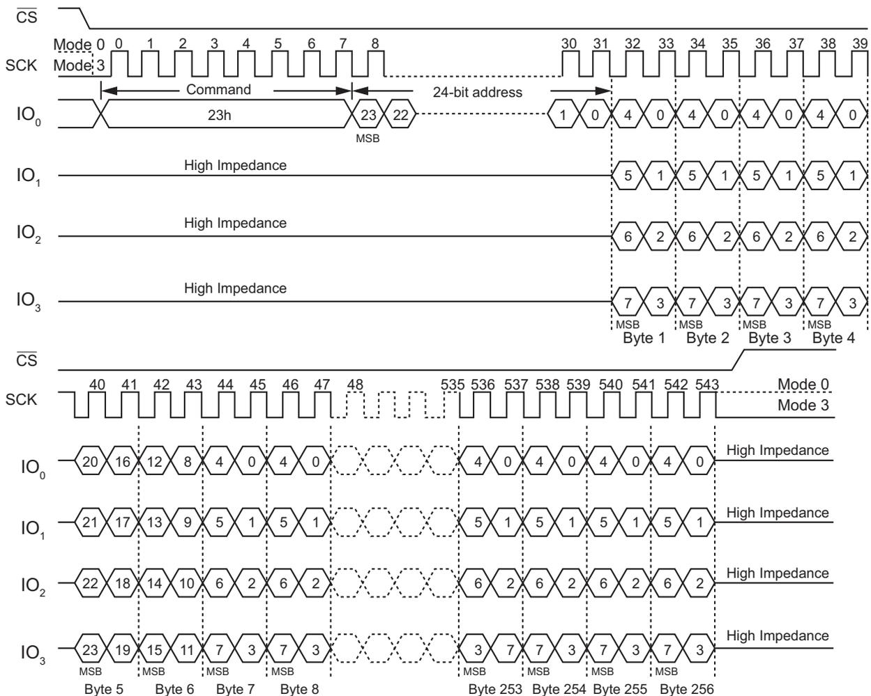
Figure 60. Quad Page Program Command (SPI mode)
