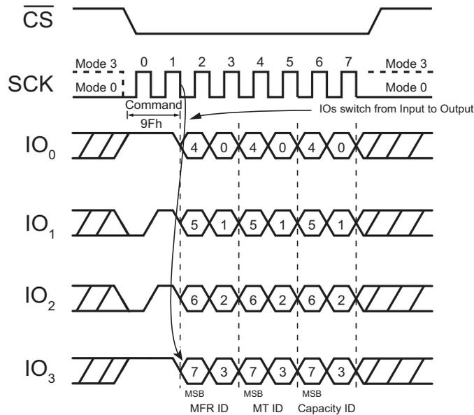
Figure 42. Read JEDEC ID Command (QPI Mode)
