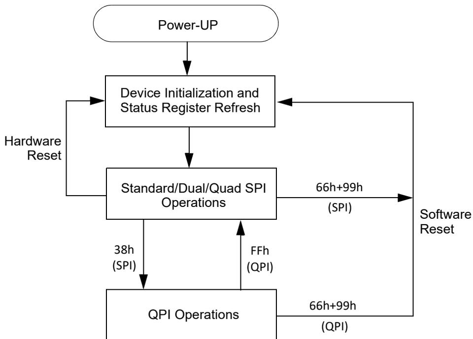
Figure 6. Switching Between SPI and QPI Operations
