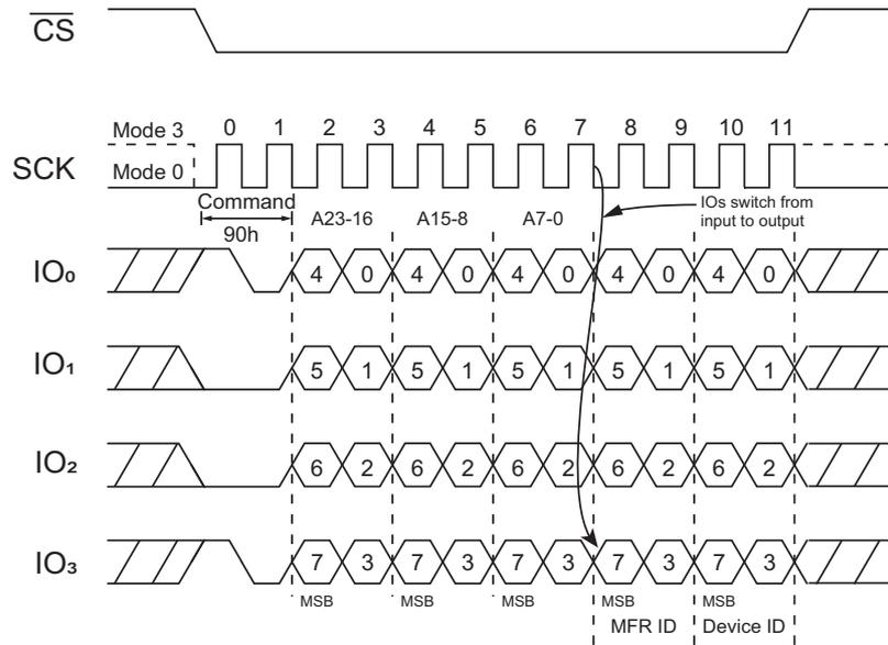
Figure 38. Read Manufacturer/ Device ID Command (QPI Mode)
