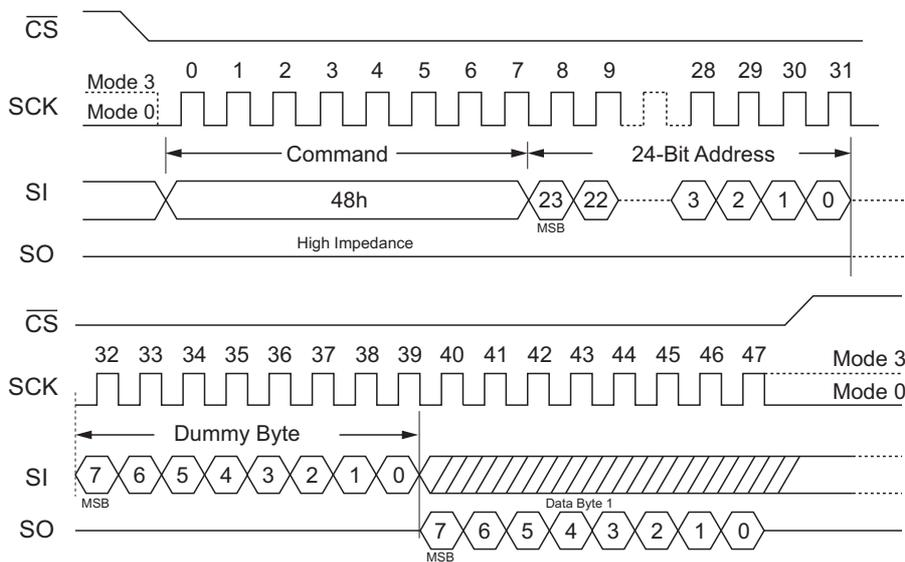
Figure 50. Read Security Register, SPI Mode
