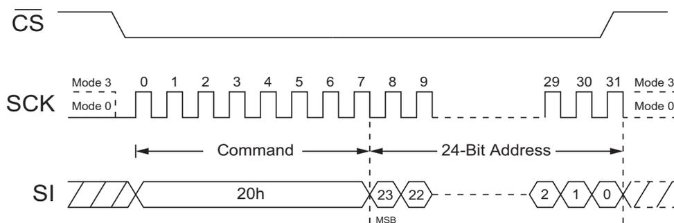
Figure 61. 4-kByte Block Erase Command (SPI Mode)
