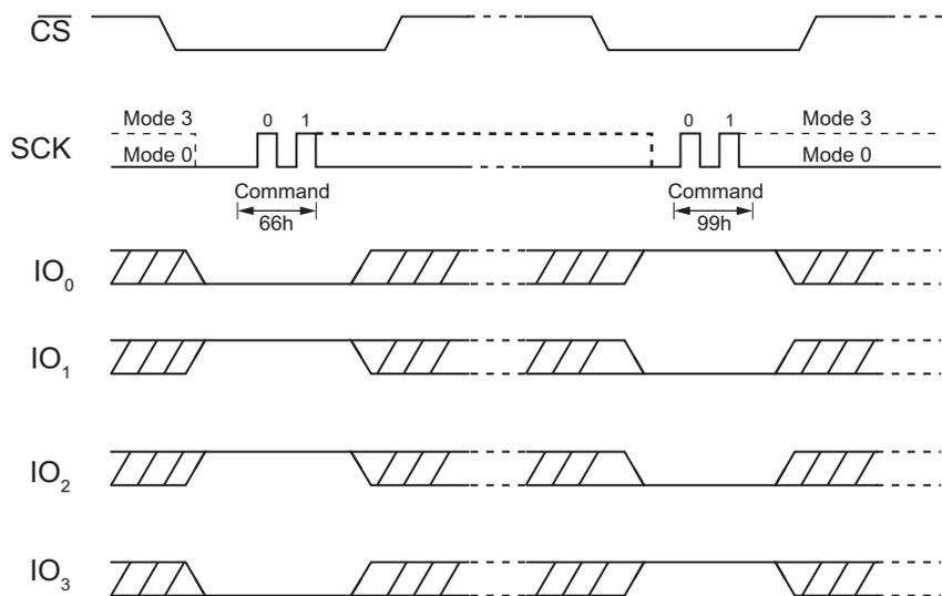
Figure 20. Enable Reset and Reset Command (QPI Mode)
