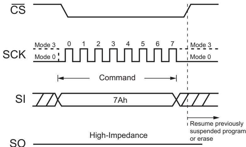
Figure 70. Erase / Program Resume Command (SPI Mode)
