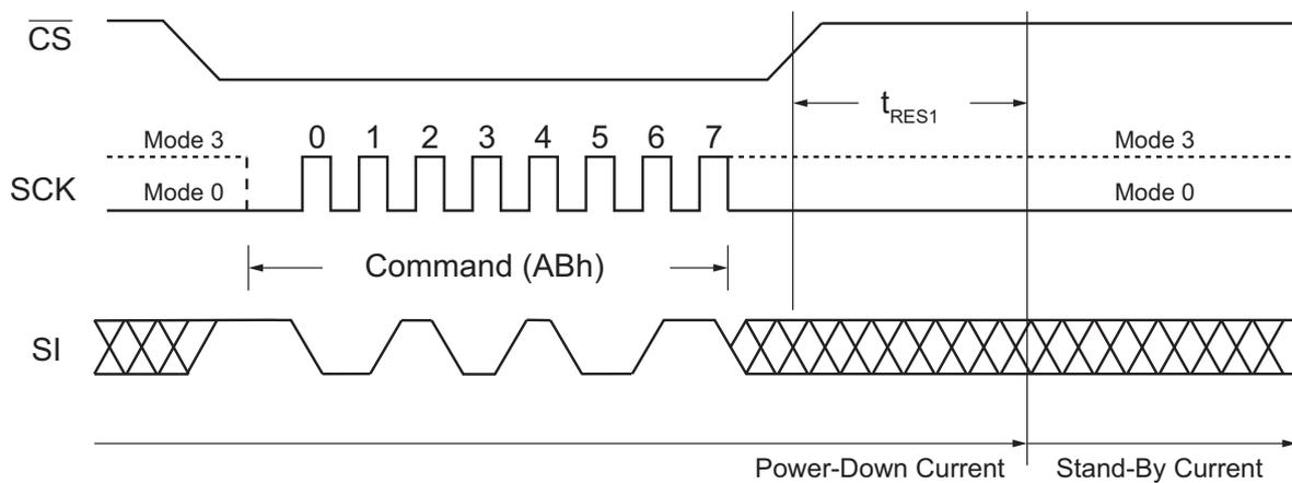
Figure 46. Release Power-Down Command (SPI Mode)
