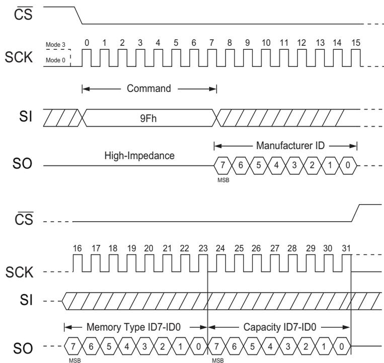
Figure 41. Read JEDEC ID Command (SPI Mode)
