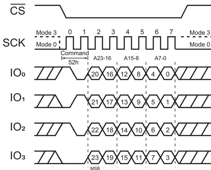
Figure 64. 32-kByte Block Erase Command (QPI Mode)
