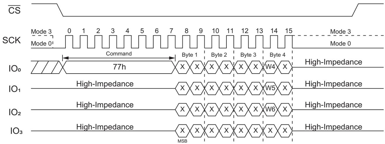
Figure 34. Set Burst with Wrap Command Sequence, SPI Only
