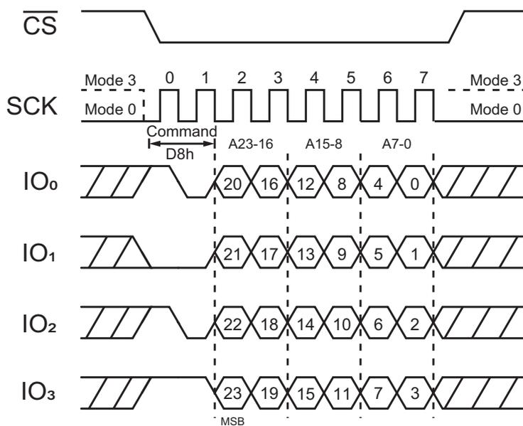
Figure 66. 64-kByte Block Erase Command (QPI Mode)
