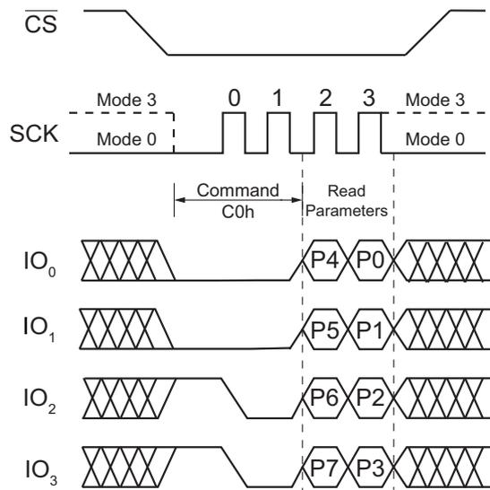
Figure 35. Set Read Parameters Command (QPI Mode)
