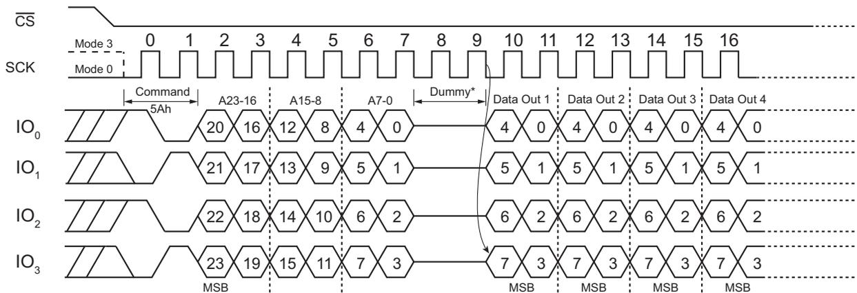
\*= "Set Read Parameters" Command(C0h) can set the number of dummy clocks
