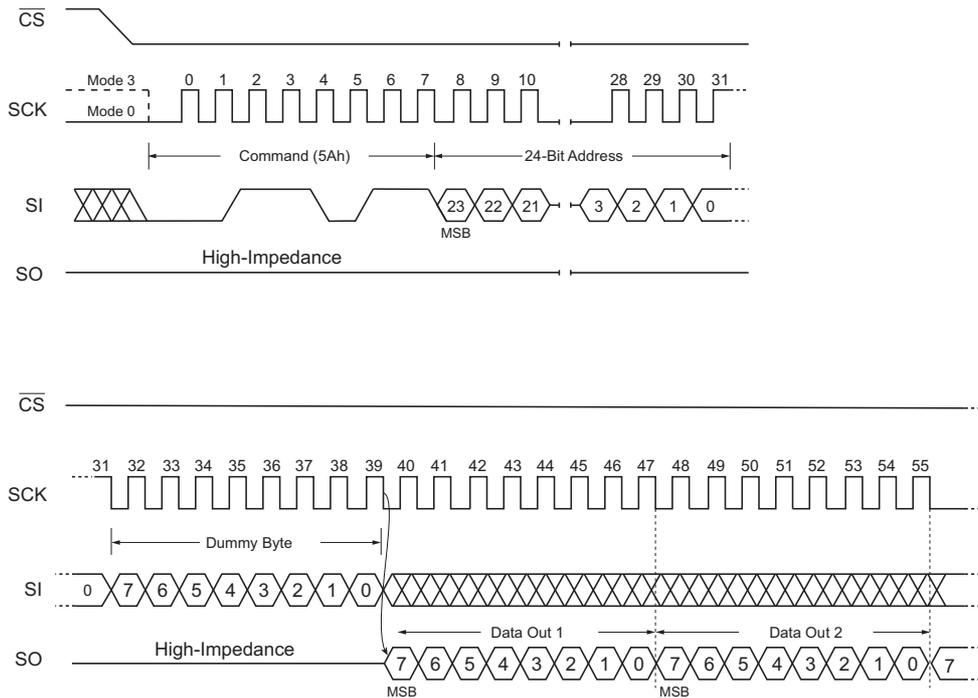
Figure 56. Read SFDP Register Command SPI Mode
