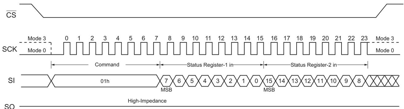
Figure 13. Write Status Register Command (SPI Mode)
