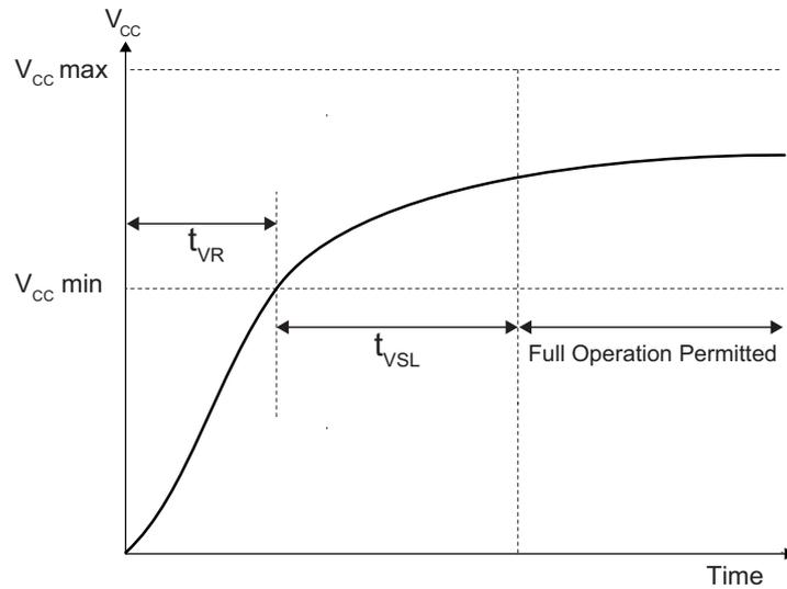
Figure 71. Power-up Timing and Voltage Levels
