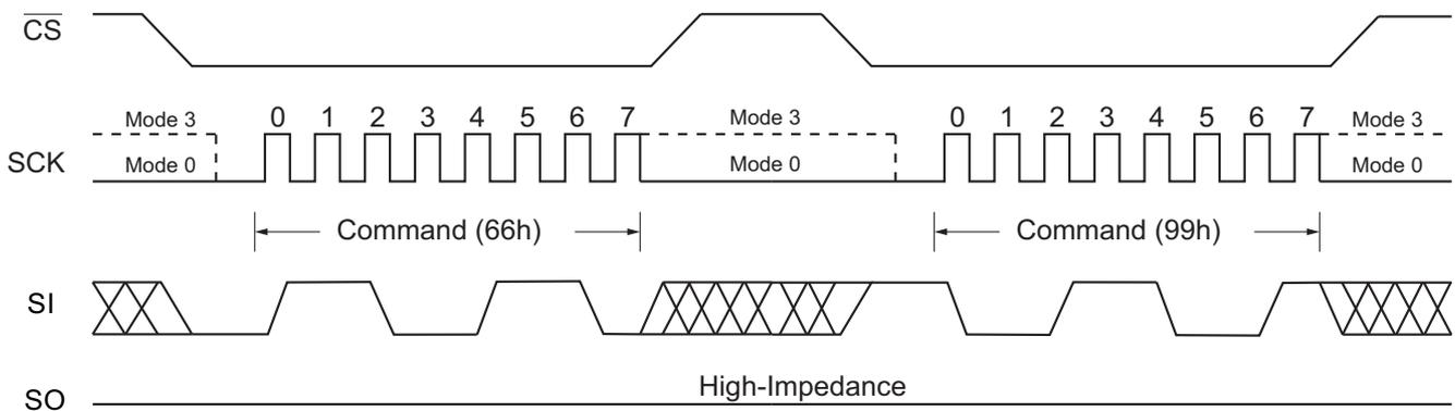
Figure 19. Enable Reset and Reset Command (SPI Mode)
