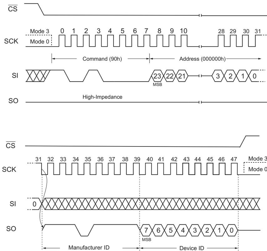
Figure 37. Read Manufacturer/ Device ID Command (SPI Mode)
