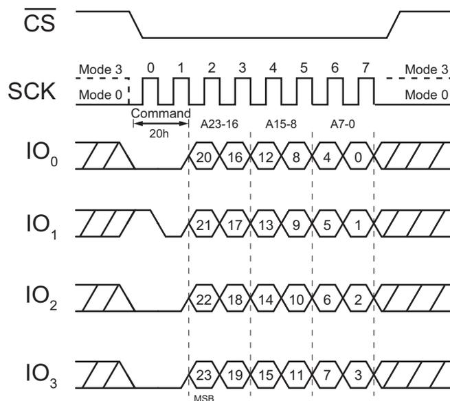
Figure 62. 4-kByte Block Erase Command (QPI Mode)
