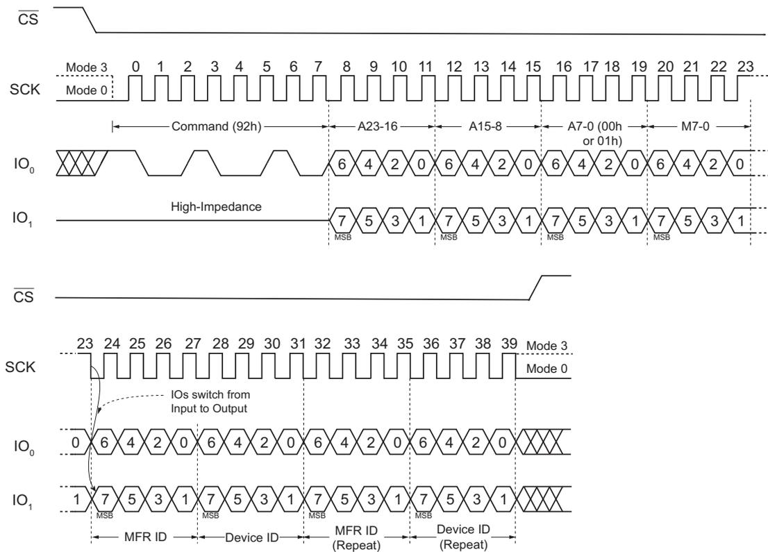
Figure 39. Read Dual Manufacturer/ Device ID Dual I/O Command (SPI Mode)
