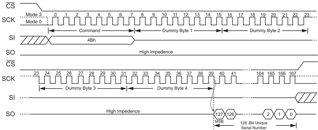
Figure 43. Read Unique ID Sequence (SPI Mode only)
