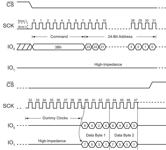
Figure 24. Fast Read Dual Output command (SPI Mode)
