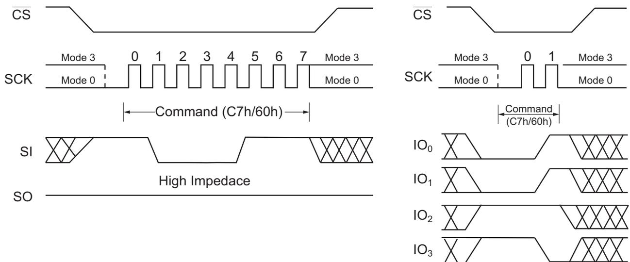
Figure 67. Chip Erase Command for SPI Mode (left) and QPI Mode (right)
