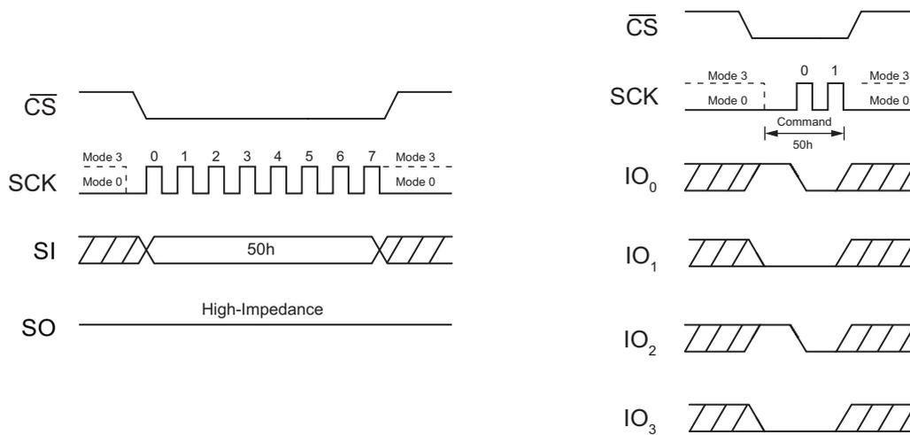
Figure 9. Write Enable for Volatile Status Register Command for SPI Mode (left) and QPI Mode (right)
