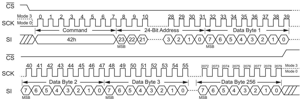
Figure 54. Program Security Register SPI Mode
