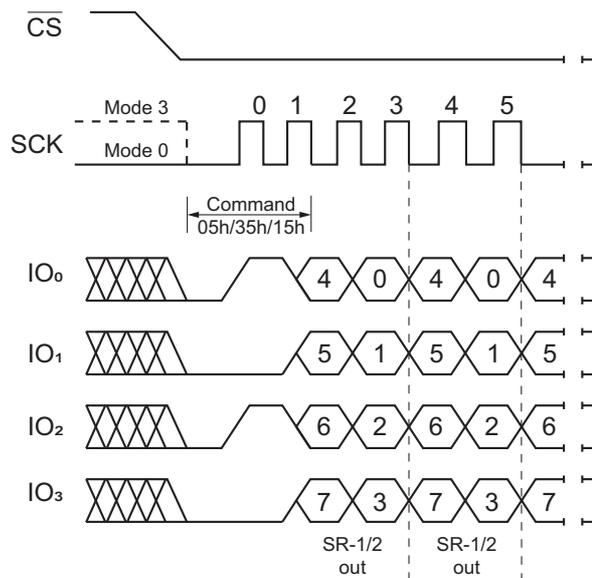
Figure 12. Read Status Register Command (QPI Mode)
