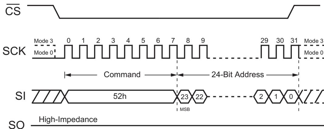
Figure 63. 32-kByte Block Erase Command (SPI Mode)
