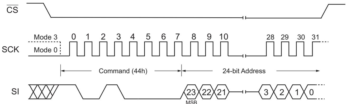
Figure 52. Erase Security Register SPI Mode
