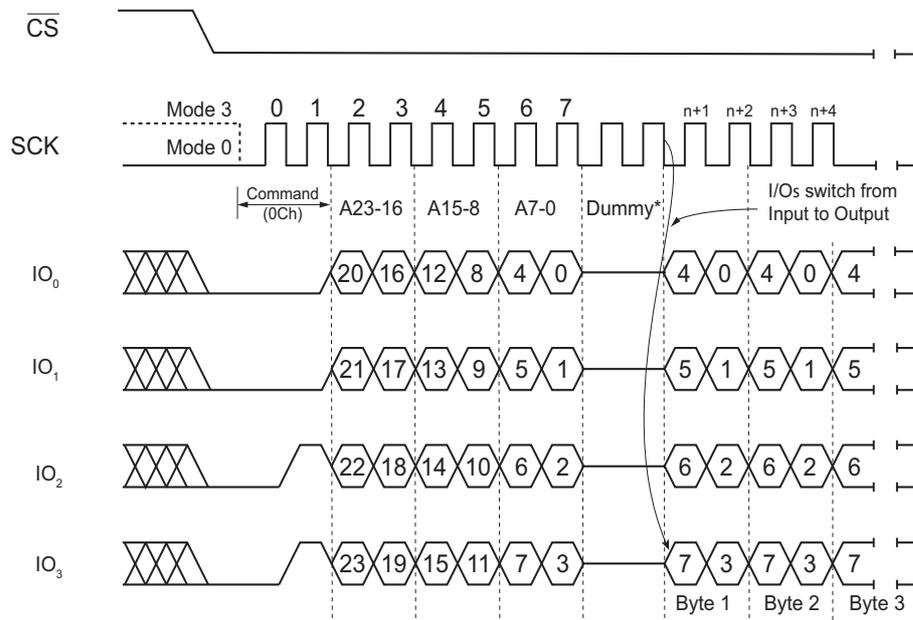
\* "Set Read Parameters" command (C0h) can set the number of dummy clocks
