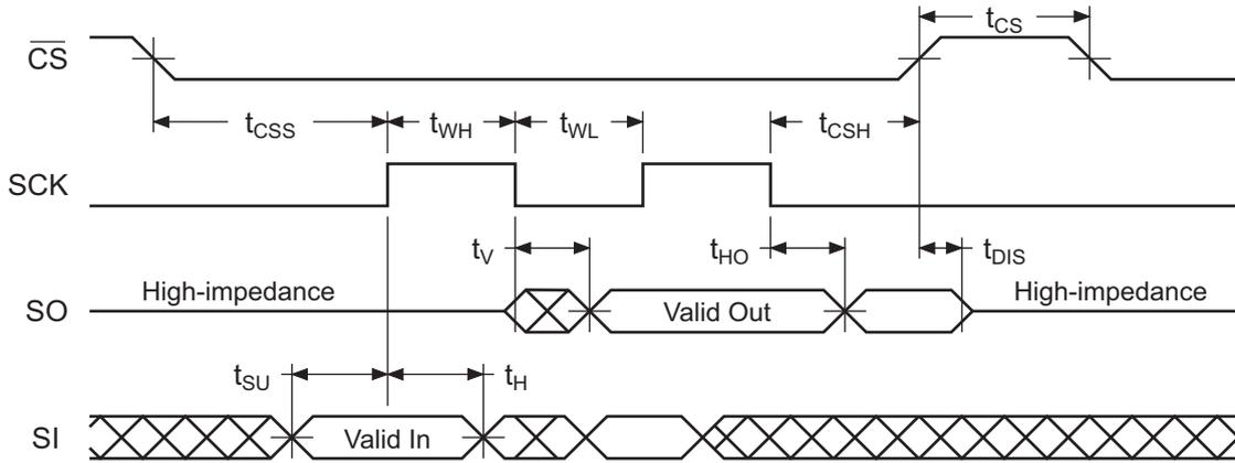
Figure 30. Waveform 1 = SPI Mode 0 Compatible
