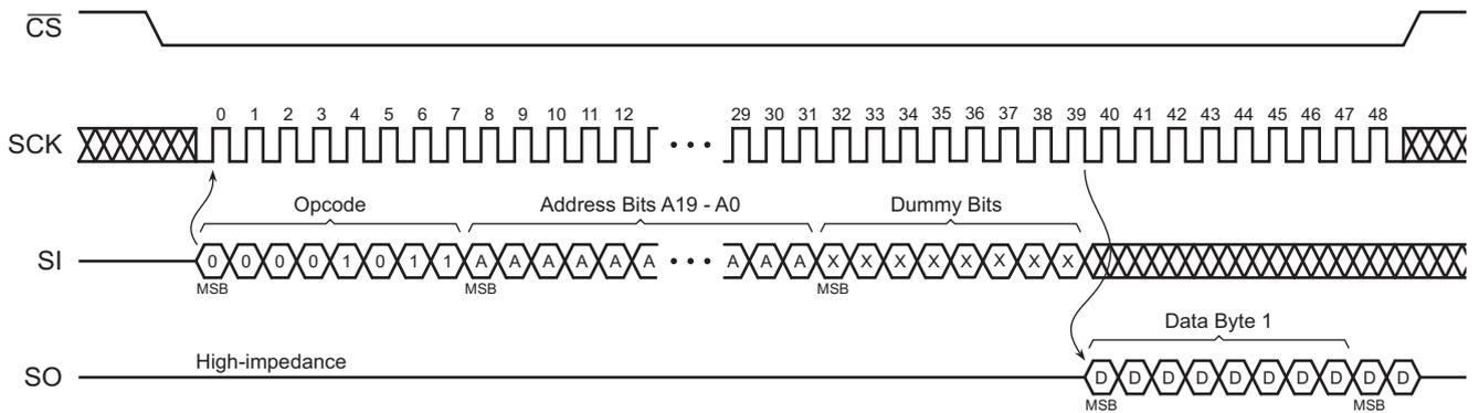
Figure 42. Continuous Array Read Timing (Opcode 0Bh)
