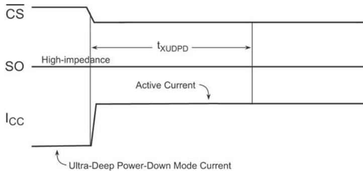
Figure 20. Exit Ultra-Deep Power-Down (Chip Select Low)
