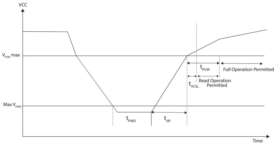
**Figure 24. Power-Up Timing**
