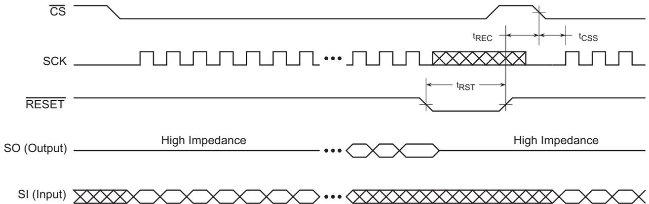
**Figure 52. Reset Timing**
