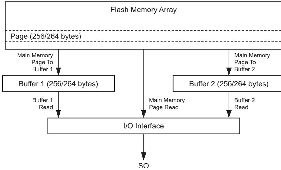
Figure 37. Block Diagram
