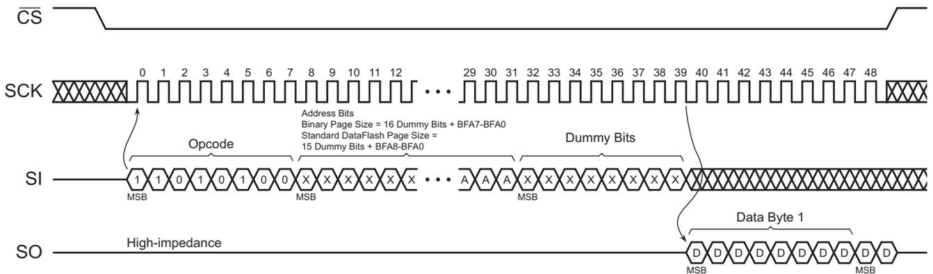
Figure 45. Buffer Read Timing (Opcode D4h or D6h)
