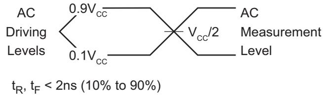
Figure 25. Input Test Waveforms and Measurement Levels
