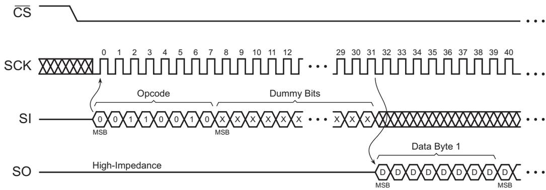
Figure 47. Read Sector Protection Register (Opcode 32h)
