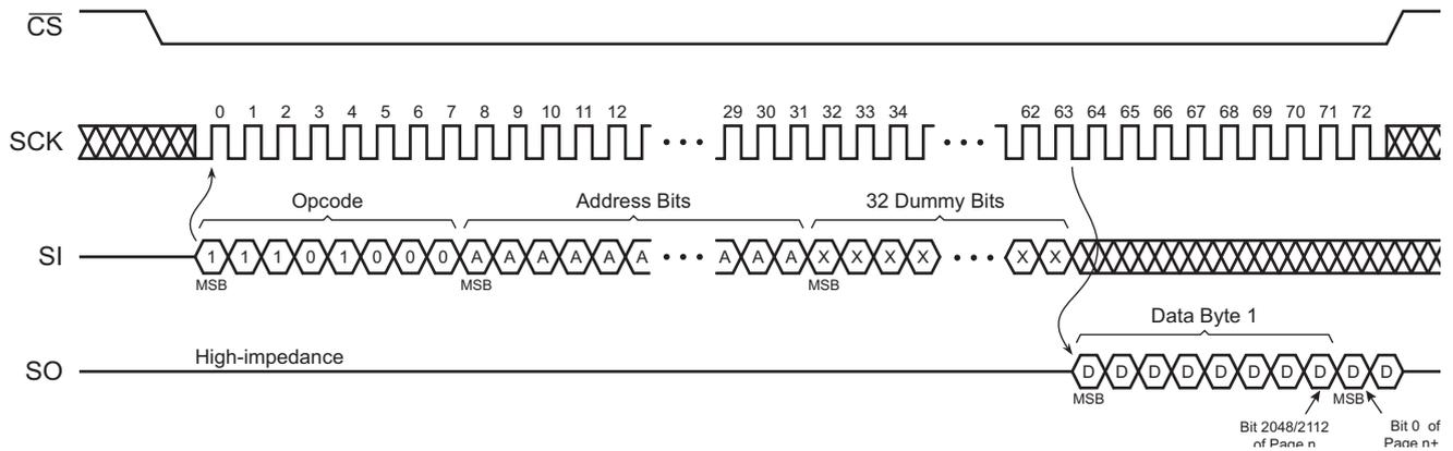
Figure 41. Continuous Array Read Timing (Legacy Opcode E8h)
