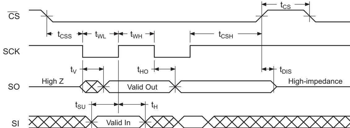
Figure 31. Waveform 2 = SPI Mode 3 Compatible
