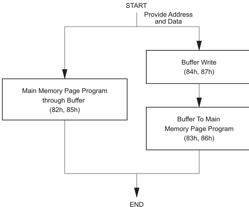
**Figure 53. Algorithm for Programming or Re-programming of the Entire Array Sequentially**
