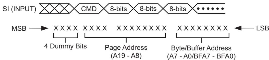
Figure 28. Command Sequence for Read/Write Operations for Page Size 256 Bytes
