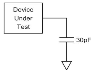
Figure 26. Output Test Load
