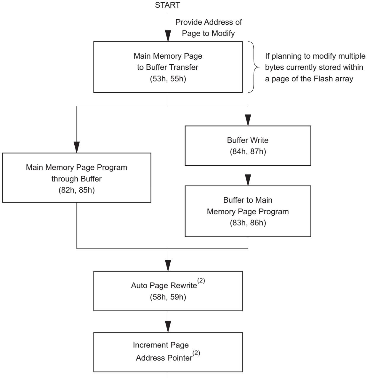
**Figure 54. Algorithm for Programming or Re-programming of the Entire Array Randomly**
