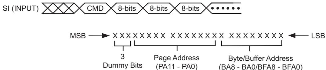
Figure 29. Command Sequence for Read/Write Operations for Page Size 264 bytes
