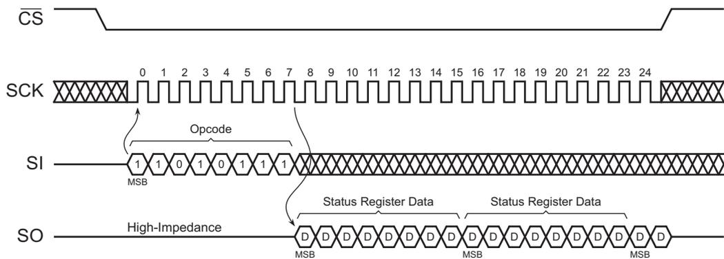
Figure 50. Status Register Read Timing (Opcode D7h)
