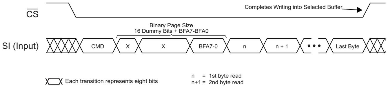
Figure 35. Buffer Write
