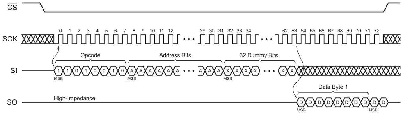
Figure 44. Main Memory Page Read Timing (Opcode D2h)
