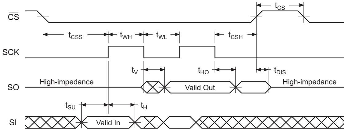
Figure 27. Waveform 1 = SPI Mode 0 Compatible
