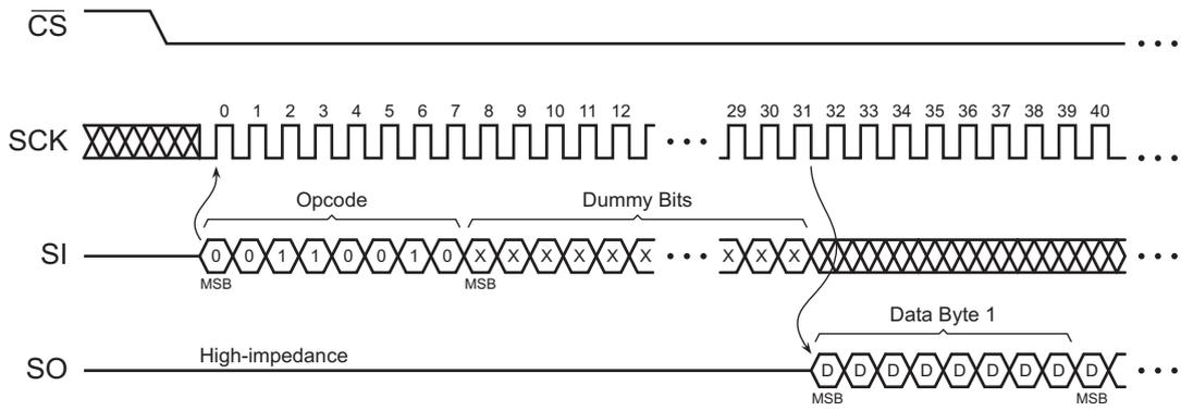
Figure 44. Read Sector Protection Register (Opcode 32h)
