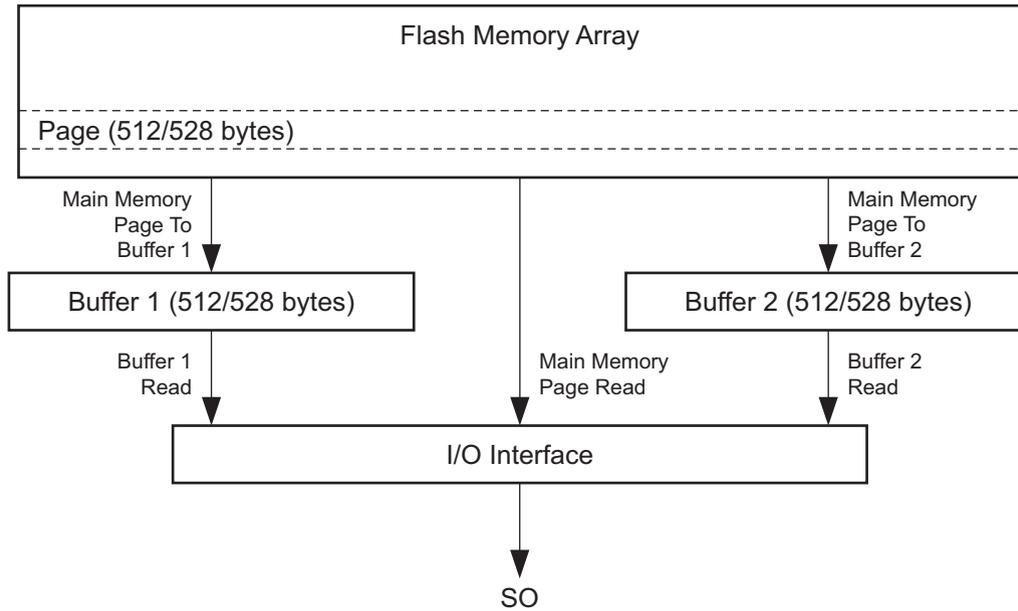
Figure 34. Block Diagram
