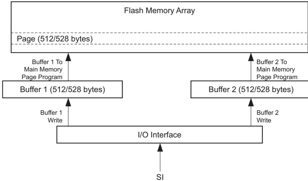
Figure 31. Block Diagram
