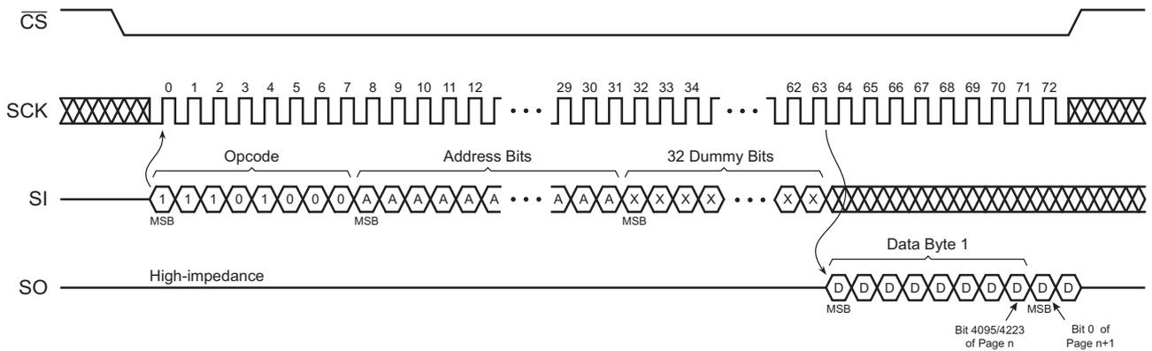
Figure 38. Continuous Array Read (Legacy Opcode E8h)
