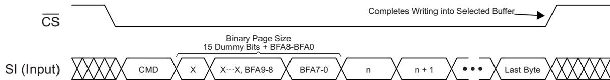
Figure 32. Buffer Write
