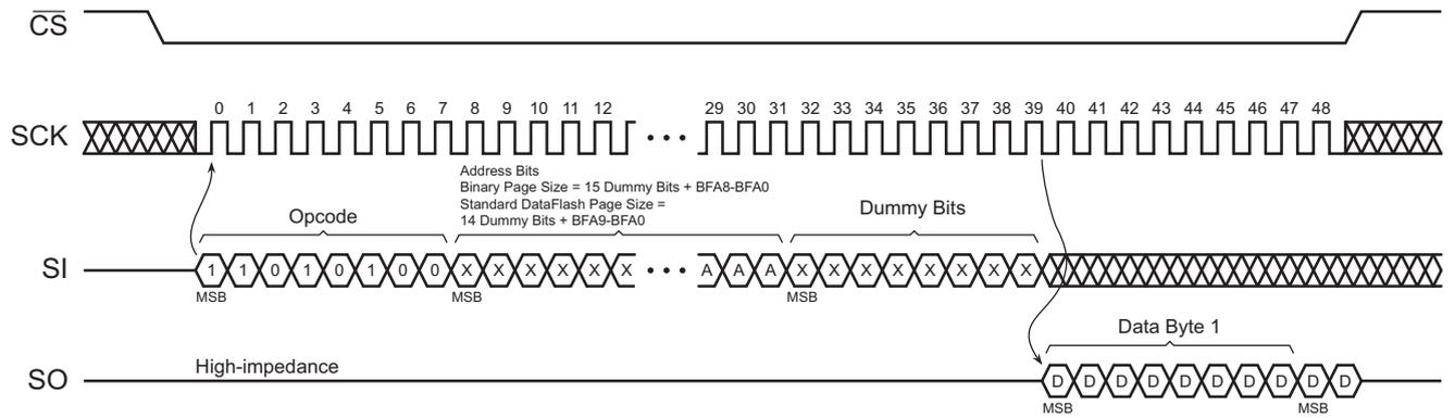
Figure 42. Buffer Read (Opcode D4h or D6h)
