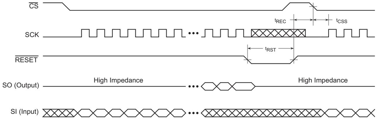
Figure 49. Reset Timing
