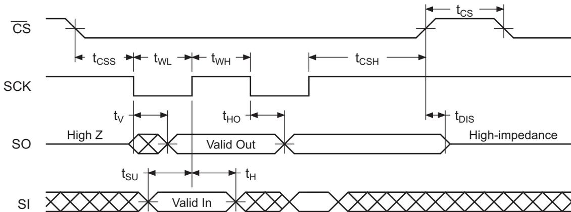
Figure 28. Waveform 2 = SPI Mode 3 Compatible
