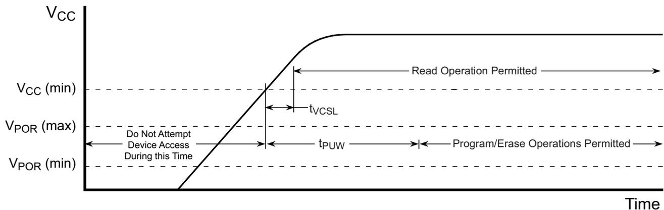
Figure 23. Power-Up Timing
