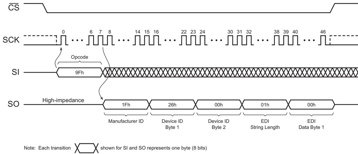
Figure 48. Manufacturer and Device Read (Opcode 9Fh)
