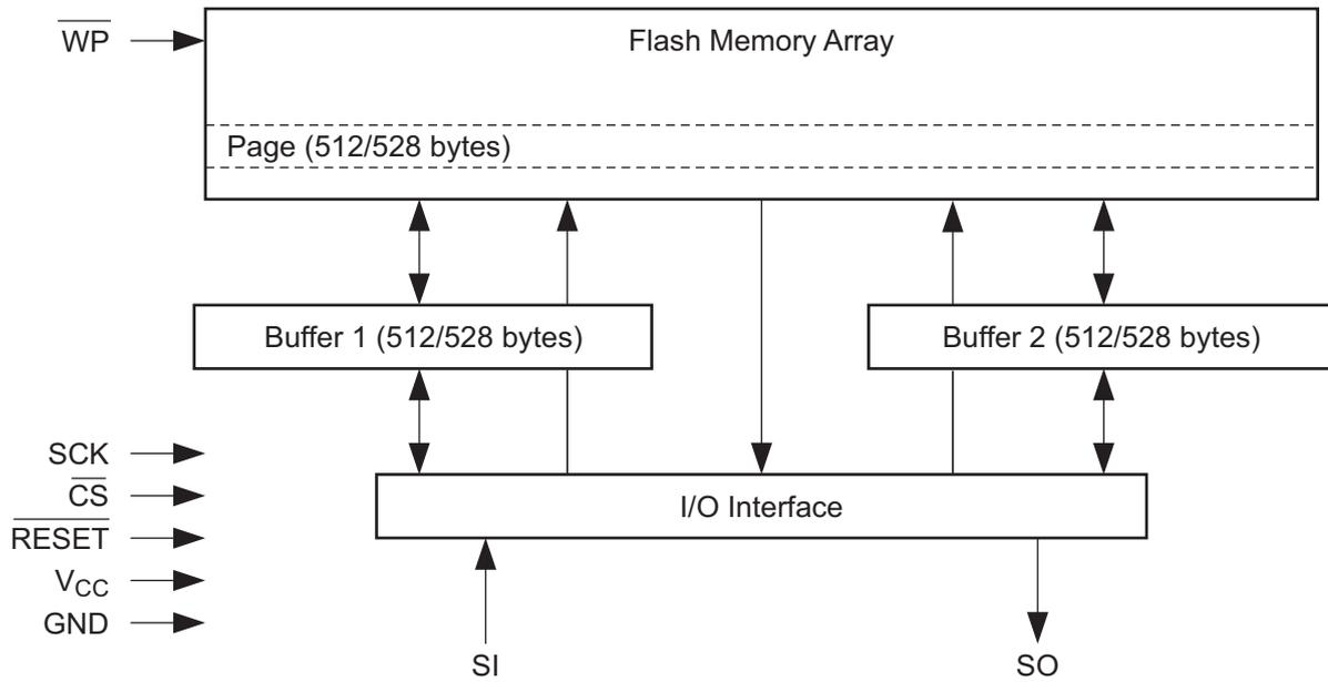
Figure 2. Block Diagram
