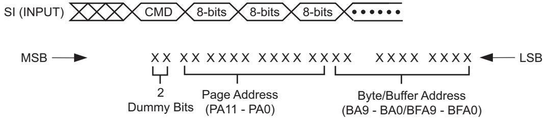
**Figure 26. Command Sequence for Read/Write Operations for Page Size 528 bytes**
