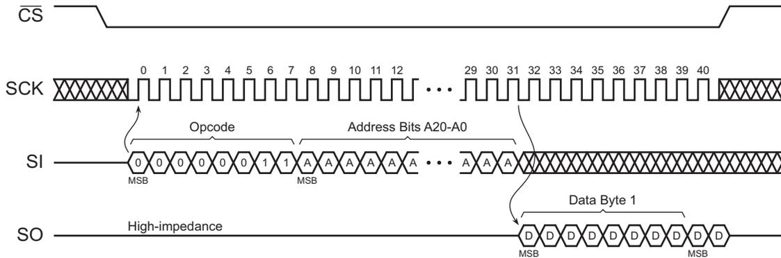
Figure 40. Continuous Array Read (Opcode 01h or 03h)
