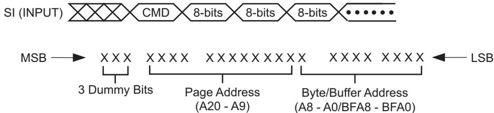
Figure 25. Command Sequence for Read/Write Operations for Page Size 512 bytes
