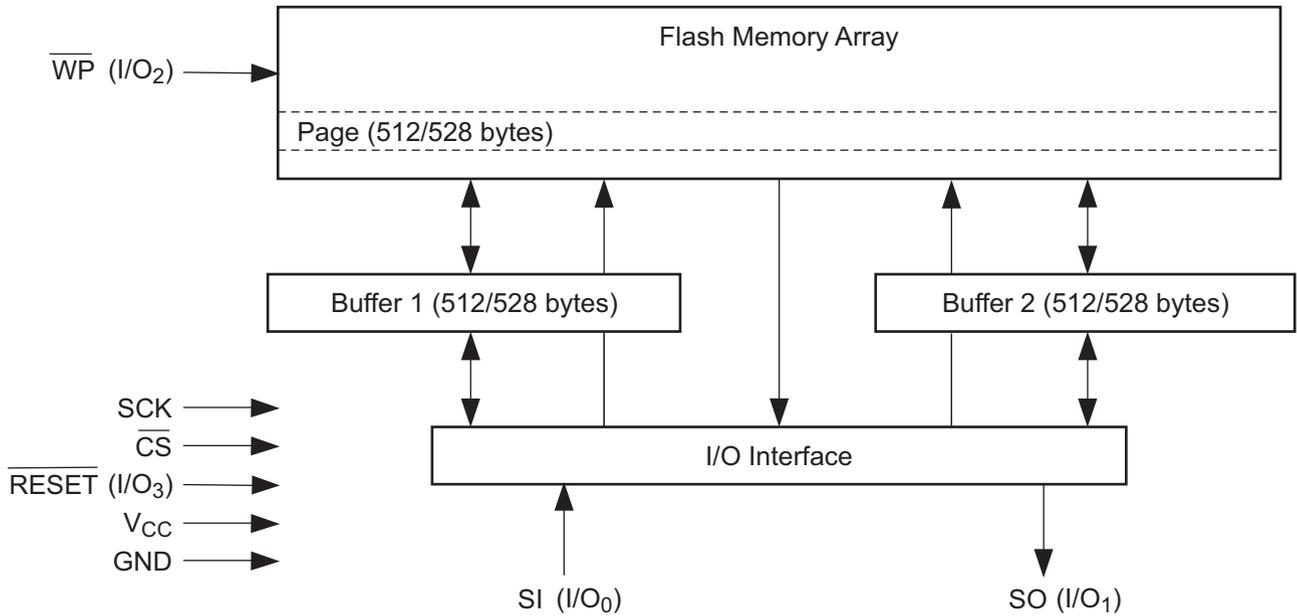
Note: I/O<sub>3-0</sub> pin naming convention is used for Dual-I/O and Quad-I/O commands.
