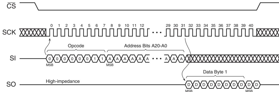
Figure 47. Continuous Array Read (Opcode 01h or 03h)
