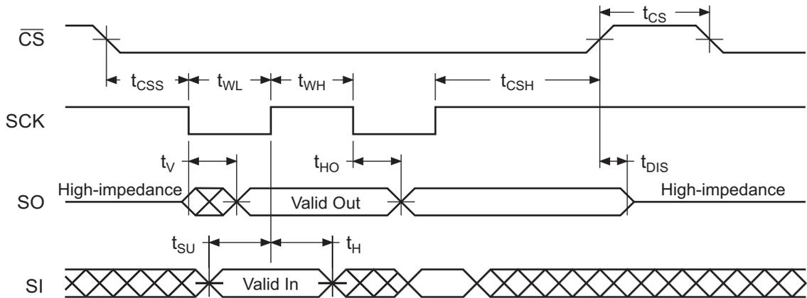
Figure 33. Waveform 2: SPI Mode 3 Compatible
