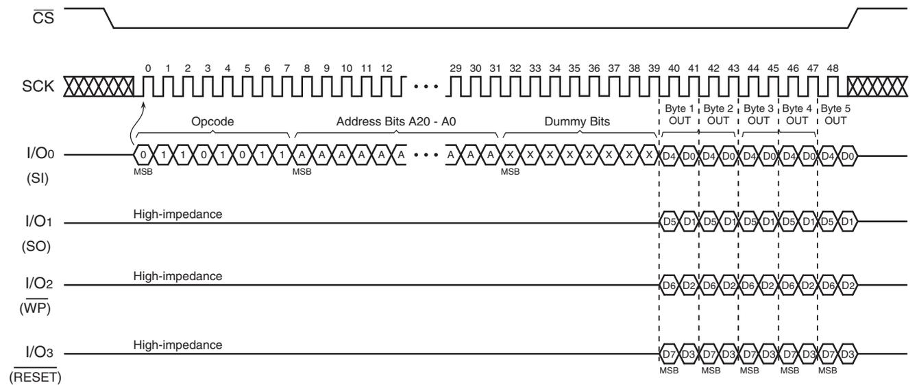
Figure 50. Quad-Output Read Array (Opcode 6Bh)
