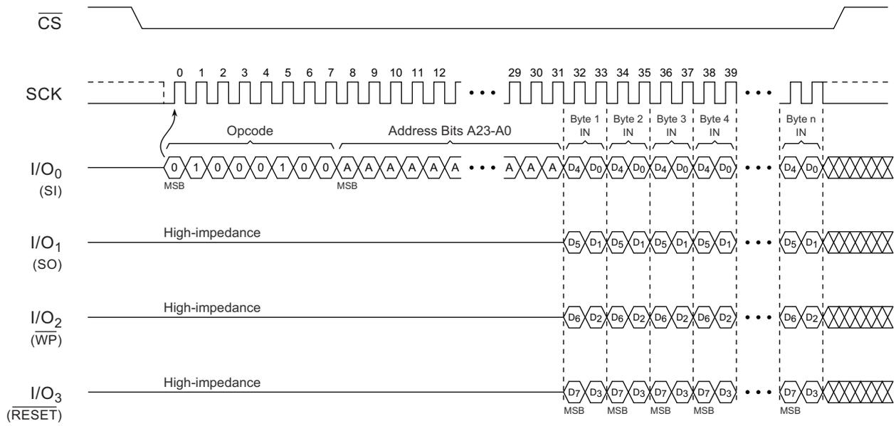
Figure 39. Quad-Input Buffer Write
