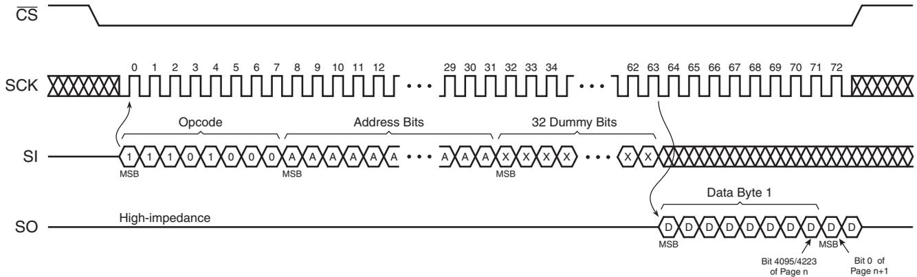
Figure 45. Continuous Array Read (Legacy Opcode E8h)
