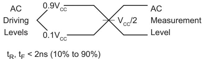
Figure 27. Input Test Waveforms and Measurement Levels
