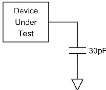
Figure 28. Output Test Load
