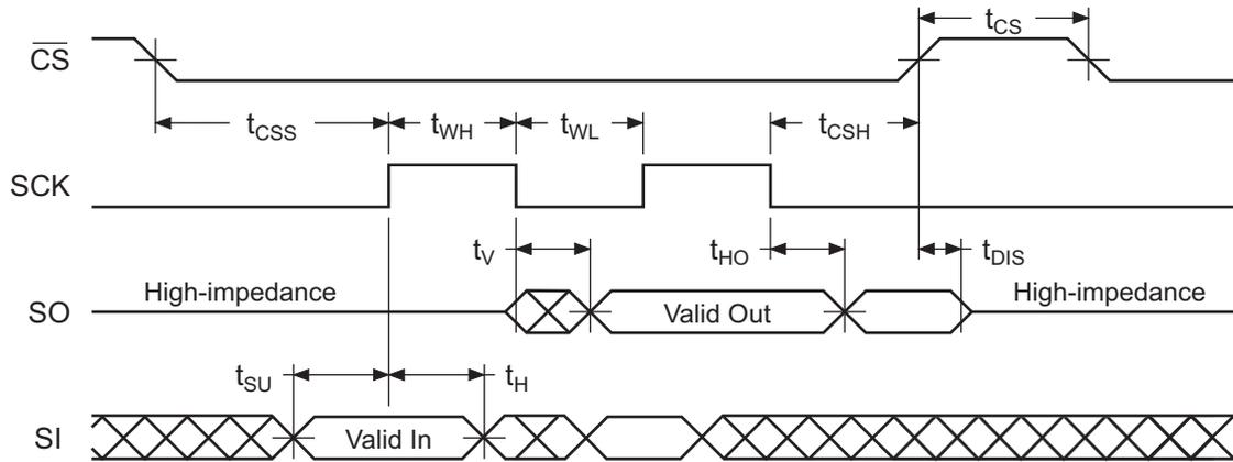
Figure 32. Waveform 1: SPI Mode 0 Compatible
