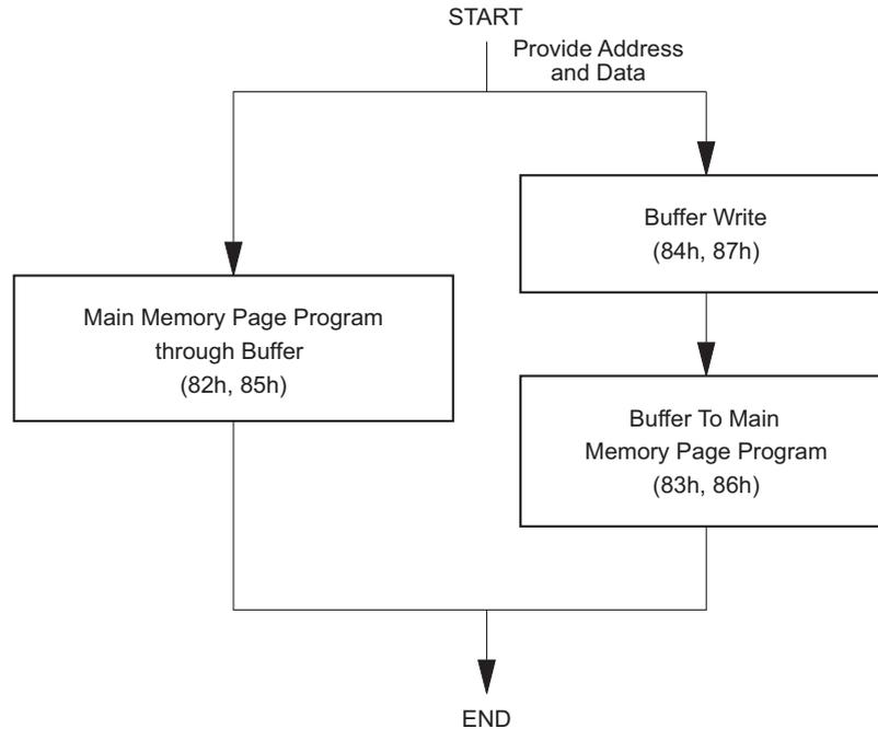
**Figure 59. Algorithm for Programming or Re-Programming of the Entire Array Sequentially**
