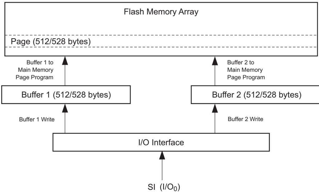
Figure 36. Block Diagram - Write
