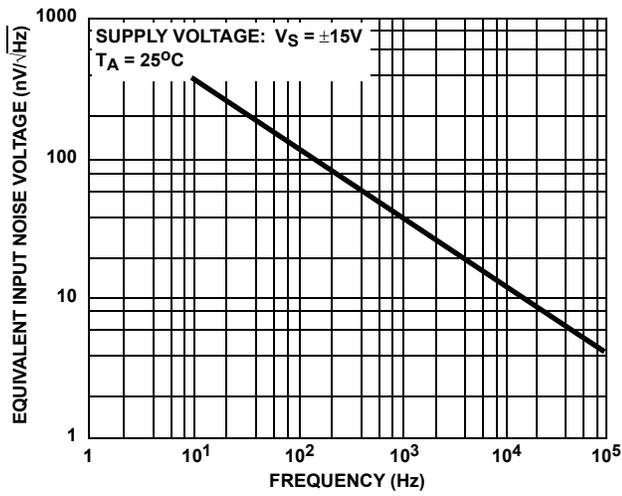
FIGURE 35. EQUIVALENT INPUT NOISE VOLTAGE vs FREQUENCY
