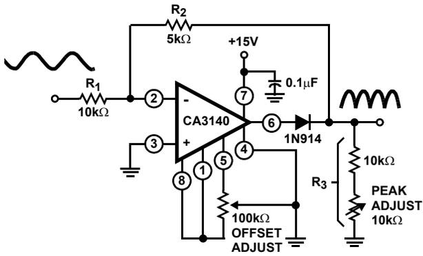
$$GAIN = \frac{R_2}{R_1} = X = \frac{R_3}{R_1 R_2 + R_3}$$
