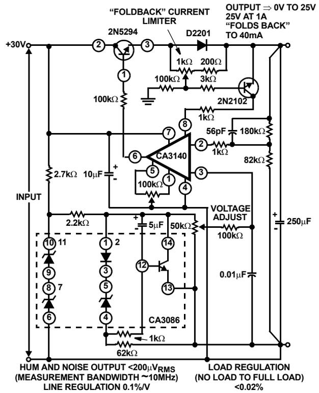
FIGURE 17. REGULATED POWER SUPPLY WITH "FOLDBACK" CURRENT LIMITING
