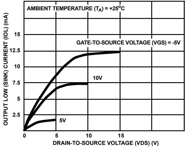
FIGURE 3. MINIMUM OUTPUT LOW (SINK) CURRENT CHARACTERISTICS
