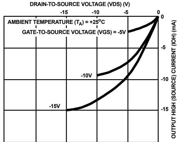
FIGURE 5. MINIMUM OUTPUT HIGH (SOURCE) CURRENT CHARACTERISTICS
