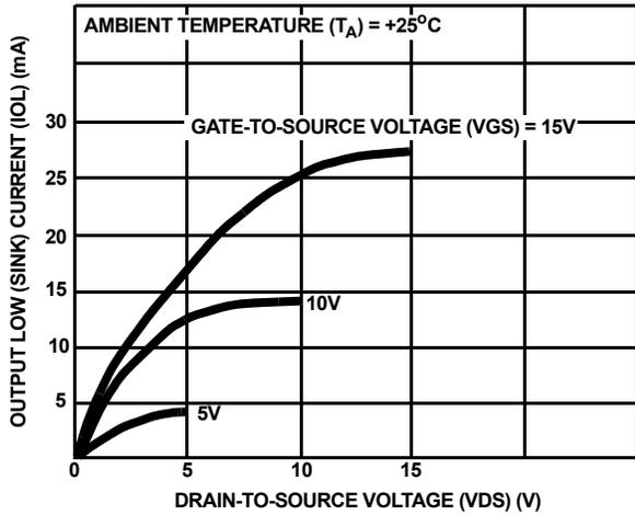
FIGURE 2. TYPICAL OUTPUT LOW (SINK) CURRENT CHARACTERISTICS
