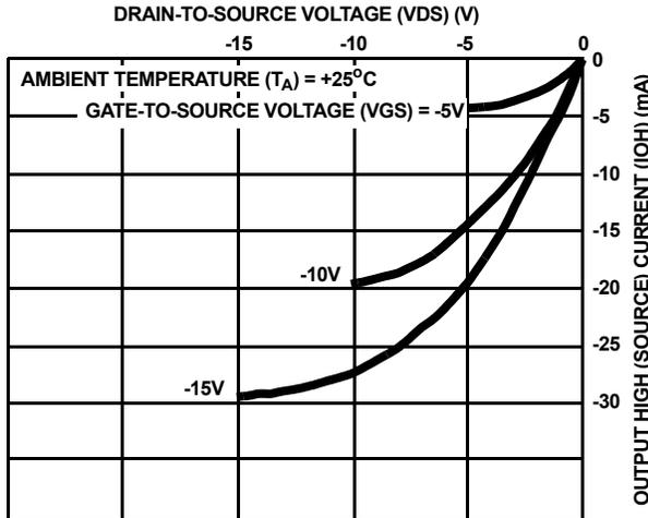
FIGURE 4. TYPICAL OUTPUT HIGH (SOURCE) CURRENT CHARACTERISTICS
