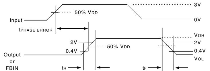
Load Circuit and Voltage Waveforms
