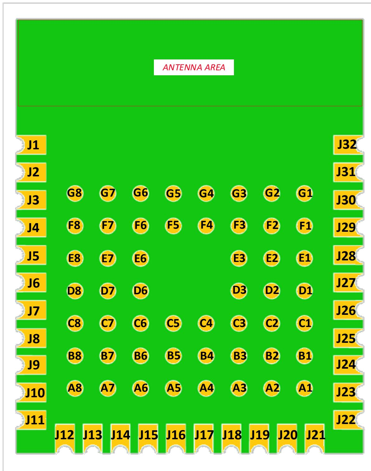
Figure 3. Pinout diagram – bottom pads (top view)
