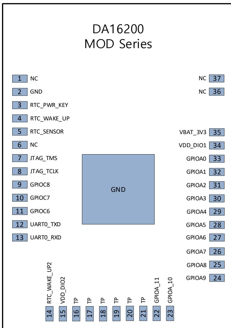
Figure 2. DA16200MOD 37 pinout diagram (top view)
