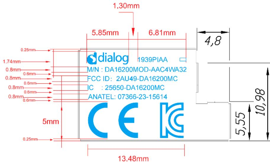
Figure 14. Physical dimensions of the module
