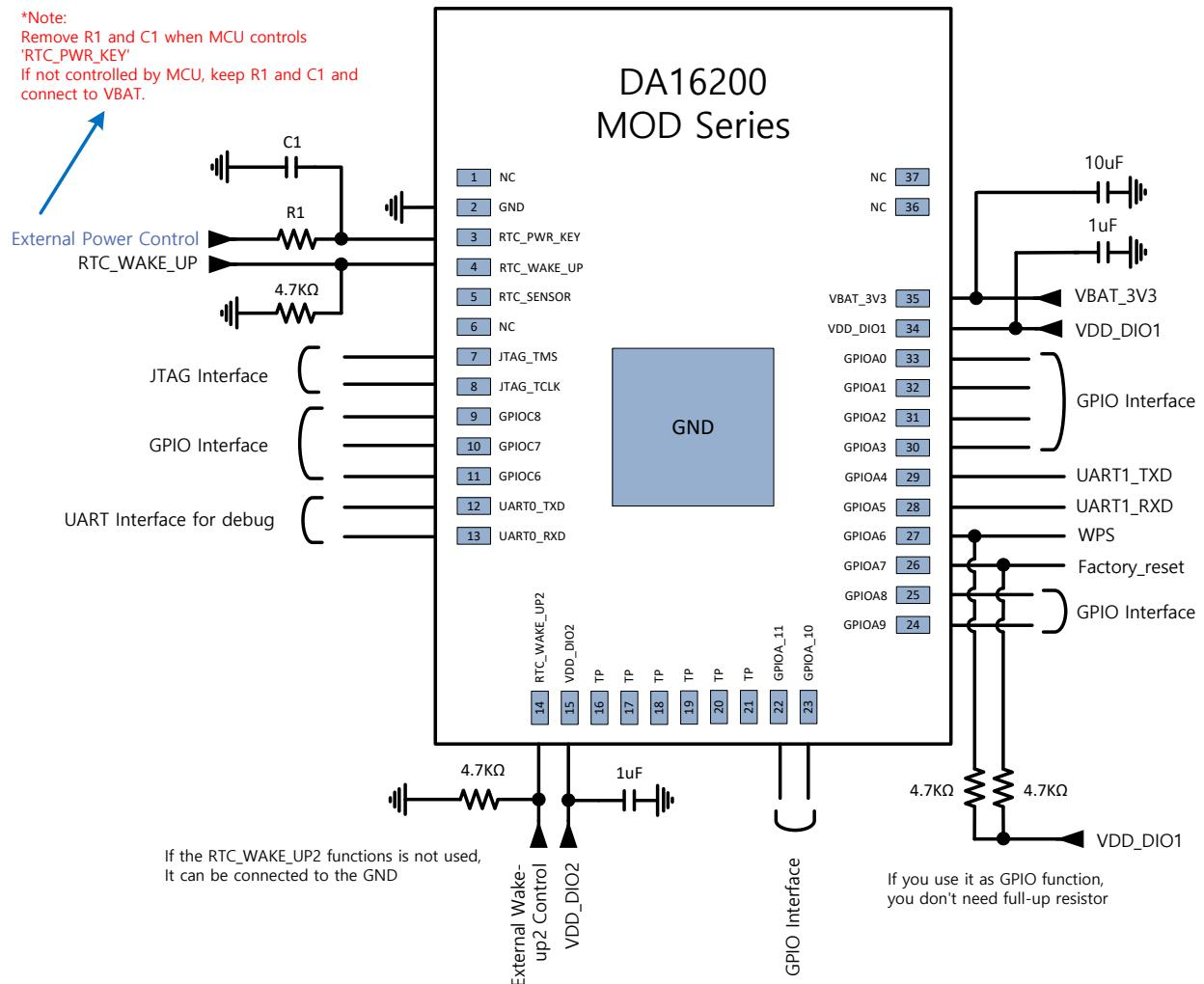
Figure 7. Application schematic
