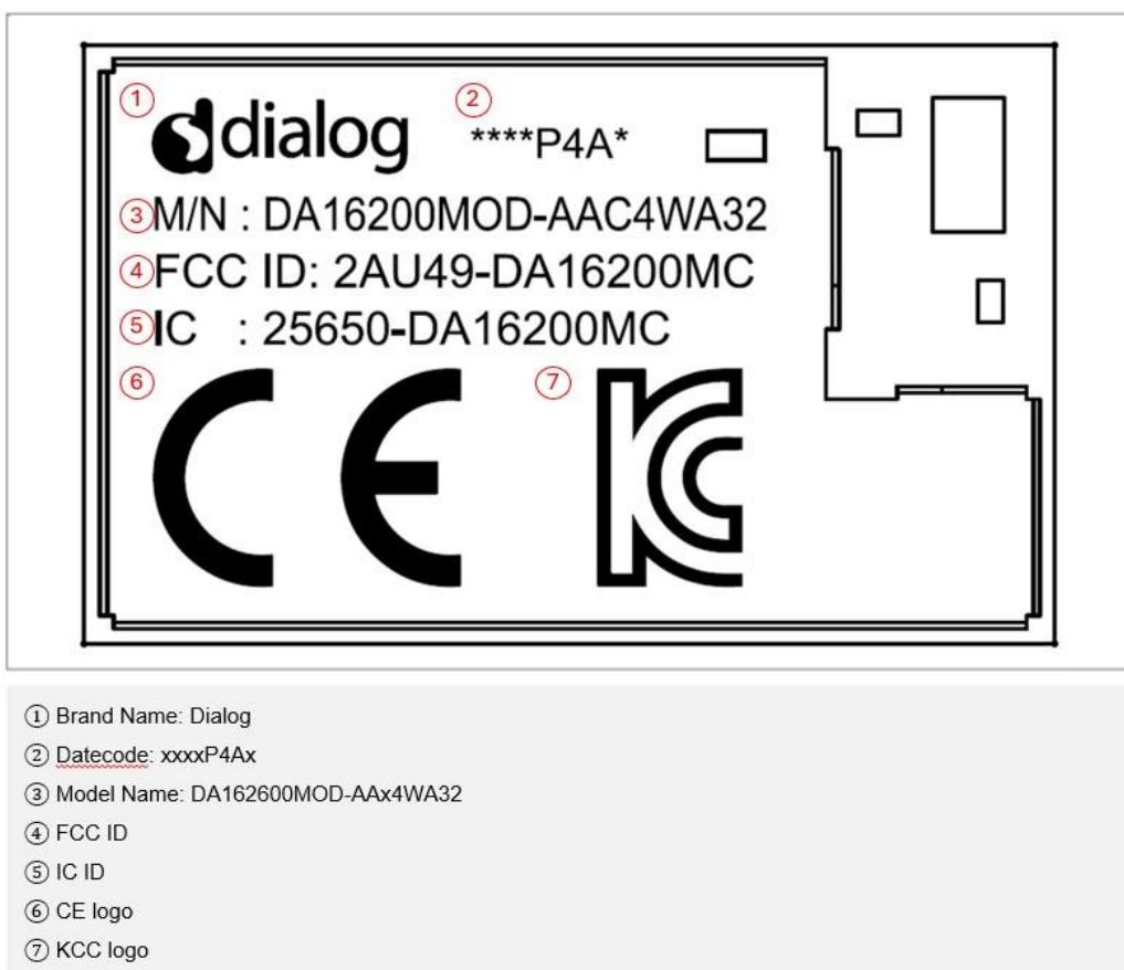
Figure 10. Module shield marking
