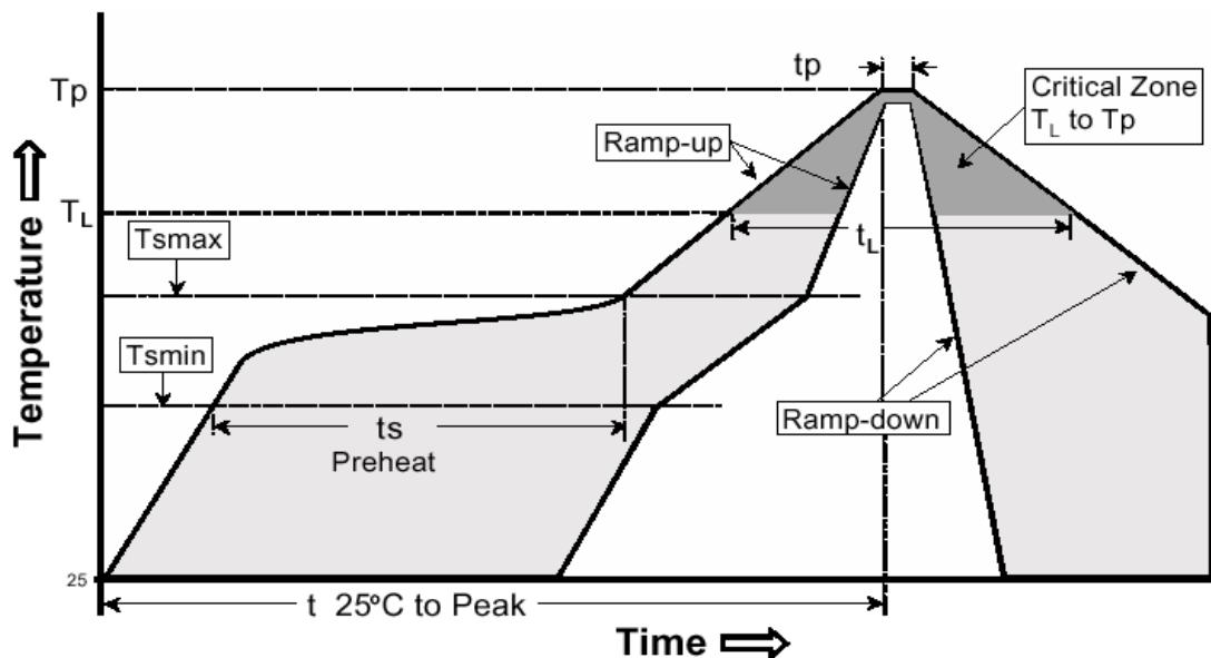
Figure 16. Reflow condition
