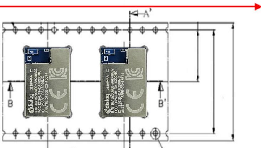
Figure 20. Component direction
