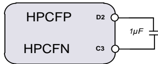
Figure 39. Charge pump flying capacitor
