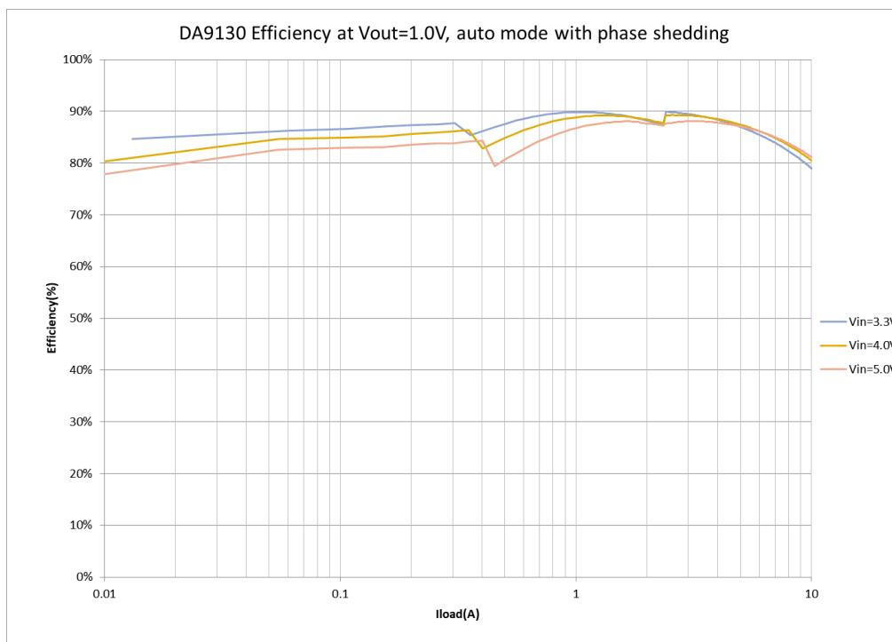
Figure 7. DA9130-A Efficiency, Auto Mode with Phase Shedding
