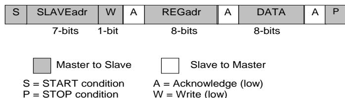
Figure 12. I<sup>2</sup>C Byte Write (SDA Line)
