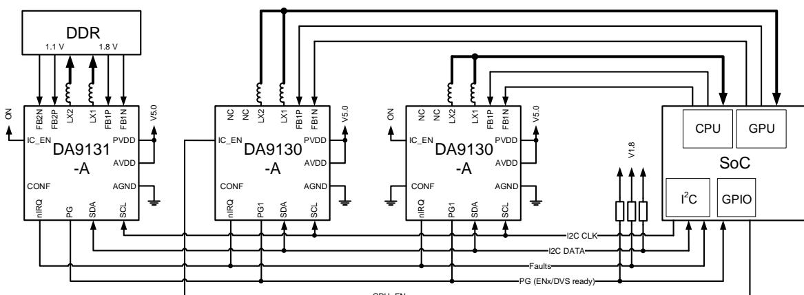
Figure 3. Typical Application Diagram (I<sup>2</sup>C Control)
