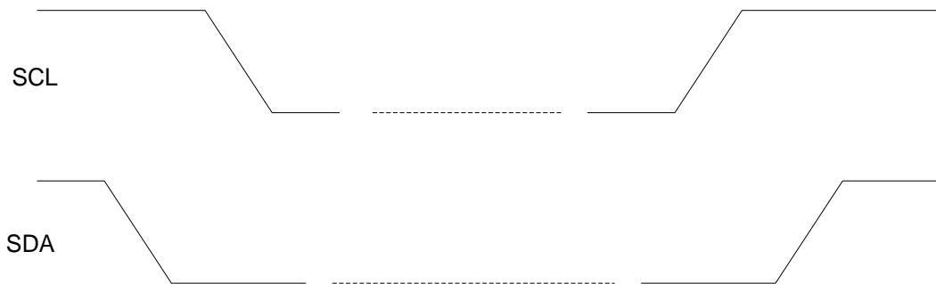
Figure 11. I<sup>2</sup>C START and STOP Condition Timing
