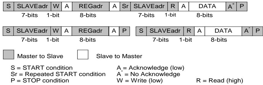
Figure 13. I<sup>2</sup>C Byte Read (SDA Line) Examples
