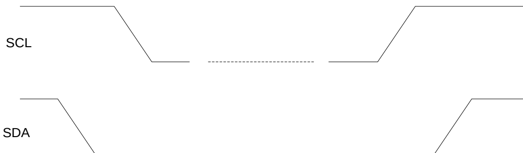
Figure 16. I 2 C START and STOP condition timing
