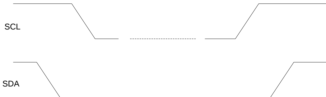
Figure 16. I 2 C START and STOP Condition Timing
