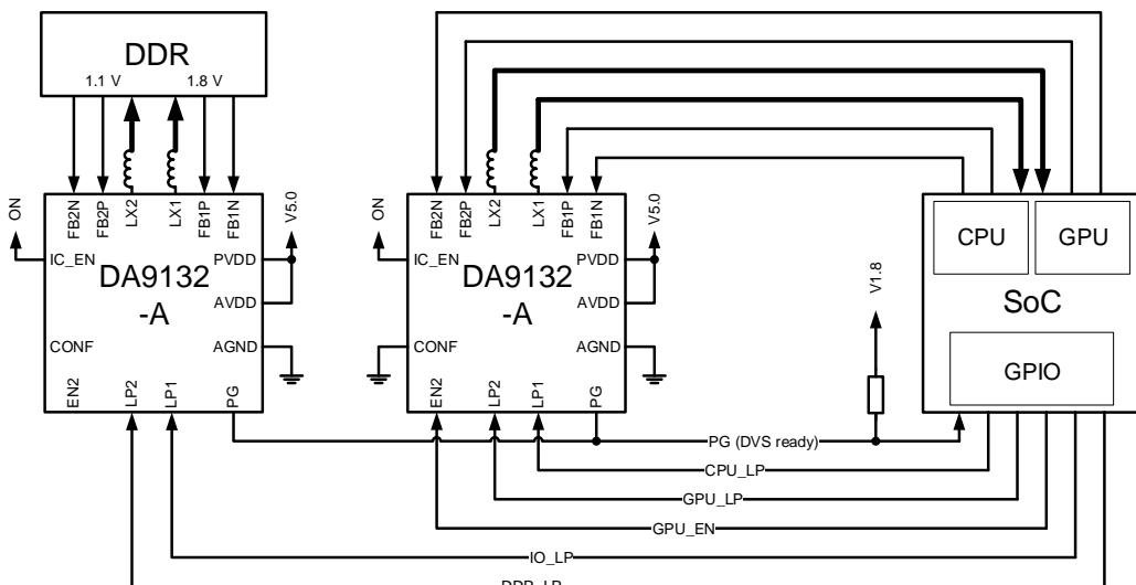
Figure 2. Typical Application Diagram (Port Control)
