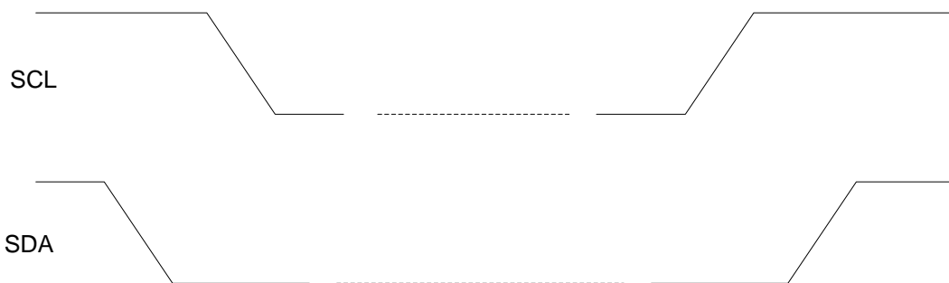
Figure 16. I 2 C START and STOP Condition Timing
