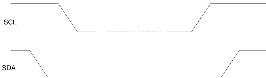
Figure 16. I<sup>2</sup>C START and STOP Condition Timing
