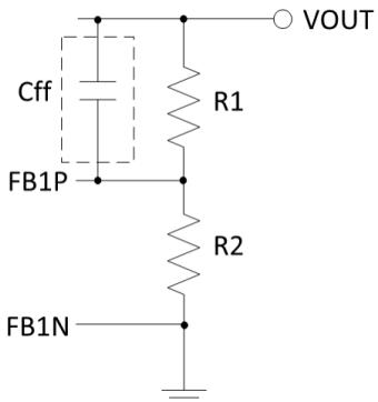
**Figure 9. Resistive Divider**
