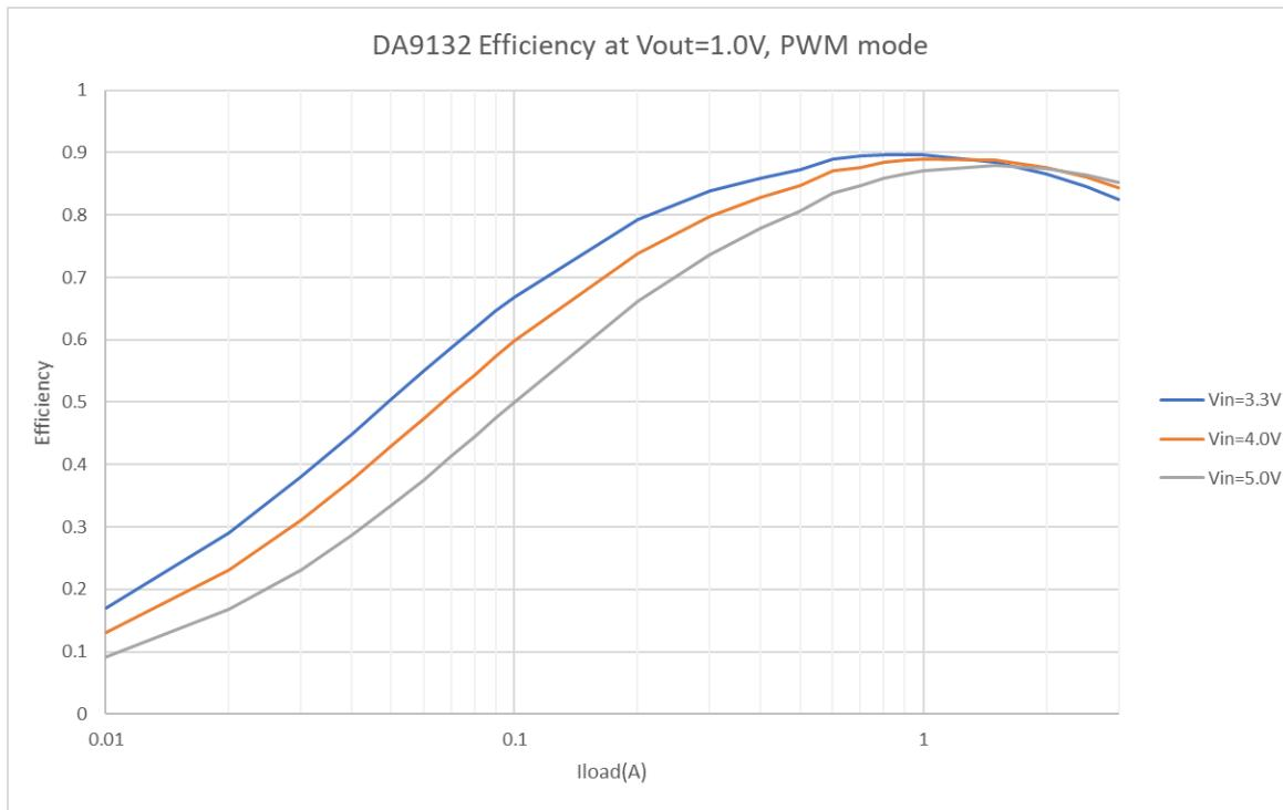
Figure 6. DA9132-A Efficiency, V<sub>OUT</sub> = 1.0 V, PWM Mode
