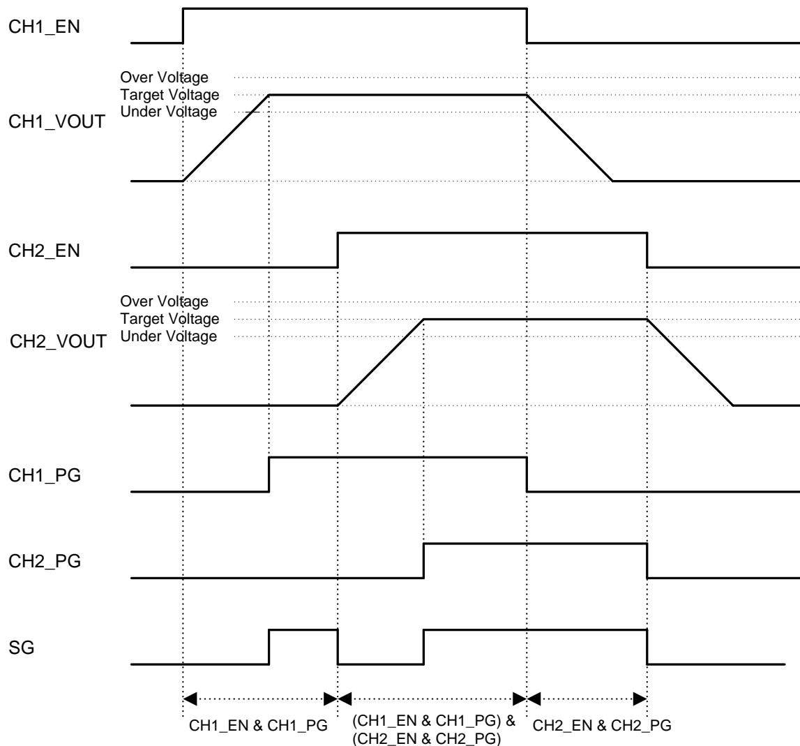
Figure 15. Power-Good (PG) and System Good (SG)
