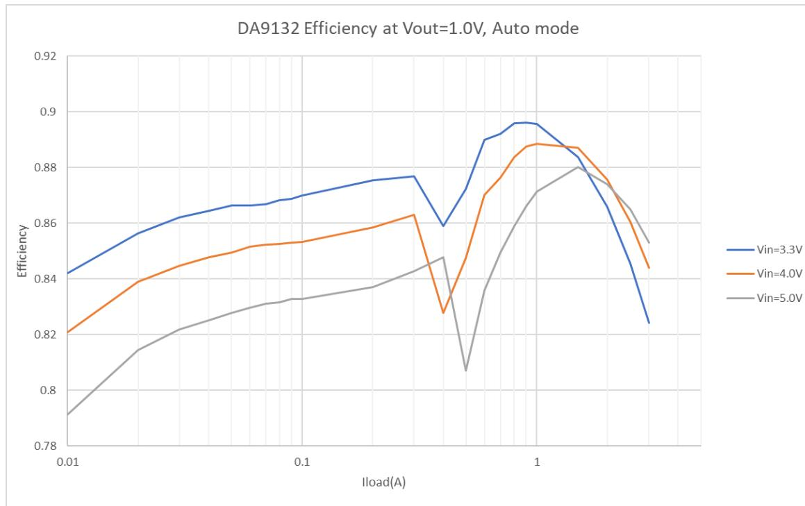
Figure 7. DA9132-A Efficiency, V<sub>OUT</sub> = 1.0 V, Auto Mode
