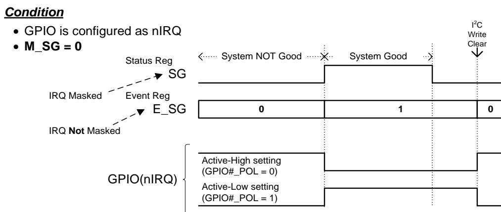
Figure 13. Interrupt Operation Example 3
