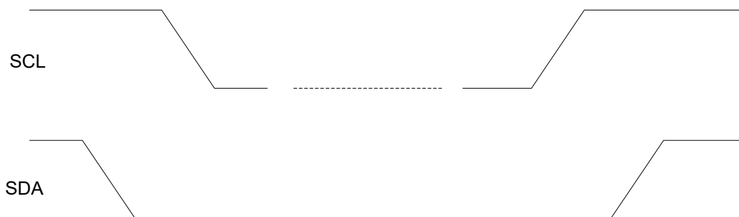
Figure 9. I 2 C START and STOP Condition Timing
