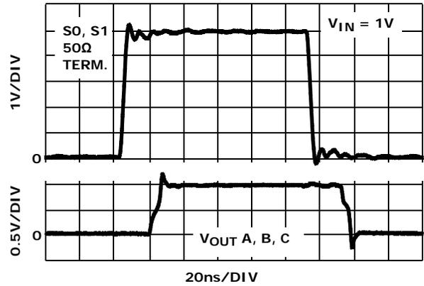
FIGURE 14. CHANNEL TO CHANNEL TRANSIENT RESPONSE  $V_{IN} = 1V$
