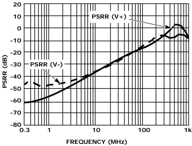
FIGURE 11. EL4340 PSRR CHANNELS A, B, C
