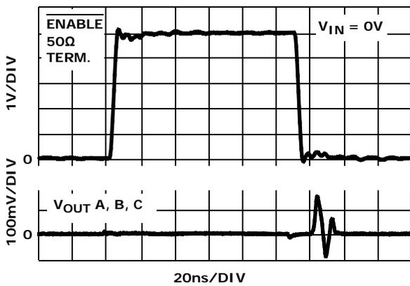
FIGURE 15. ENABLE SWITCHING GLITCH  $V_{IN} = 0V$
