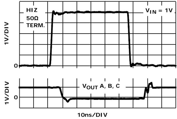
FIGURE 18. HIZ TRANSIENT RESPONSE  $V_{IN} = 1V$
