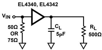
FIGURE 22A. TEST CIRCUIT WITH OPTIMAL OUTPUT LOAD
