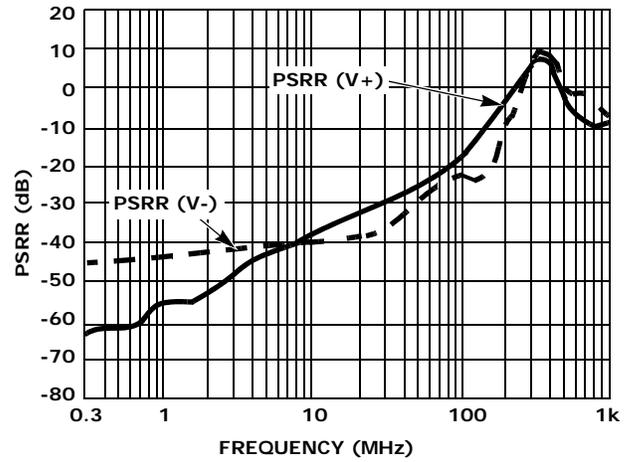
FIGURE 12. EL4342 PSRR CHANNELS A, B, C
