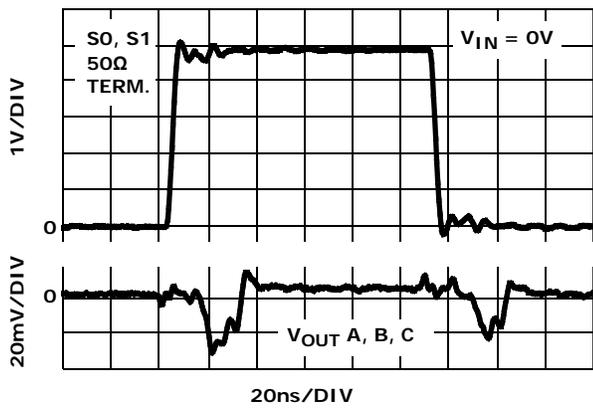
FIGURE 13. CHANNEL TO CHANNEL SWITCHING GLITCH  $V_{IN} = 0V$
