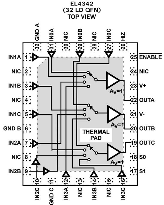
THERMAL PAD INTERNALLY CONNECTED TO V-.
