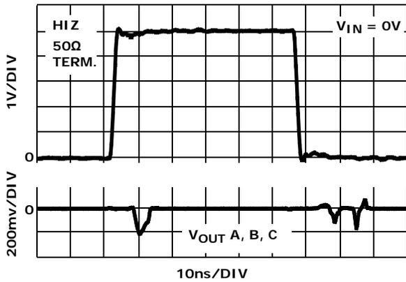
FIGURE 17. HIZ SWITCHING GLITCH  $V_{IN} = 0V$
