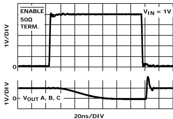
FIGURE 16. ENABLE TRANSIENT RESPONSE  $V_{IN} = 1V$
