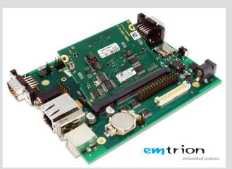
The starting point is easy. The development kit from Emtrion includes a screen, Base-Board, BSP and a DIMM module. Then once development of software is started, customers can then simply replace the base board with their own optimised base board and go into mass production. The mechanism provides a much faster time to market for all processor based systems.
