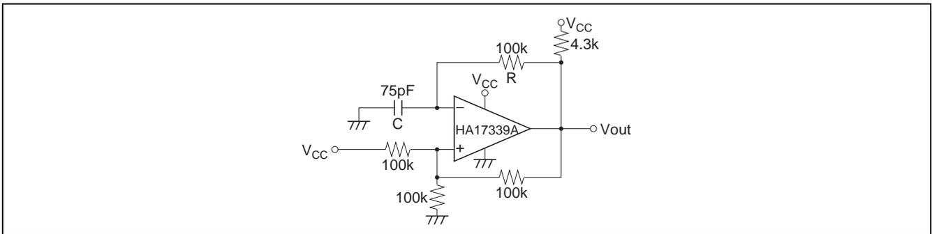
Figure 1 Square-Wave Oscillator
