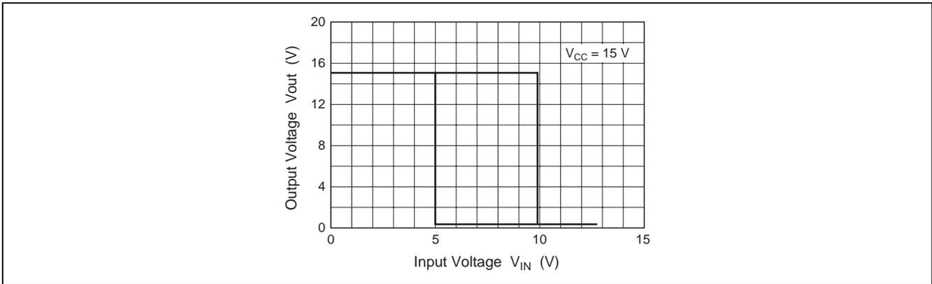
Figure 10 Inverting Comparator I/O Transfer Characteristics
