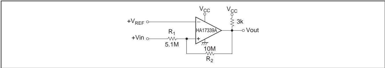
Figure 7 Noninverting Comparator
