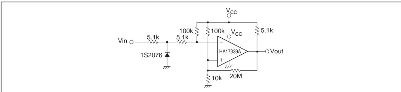
Figure 11 Zero-Cross Detector
