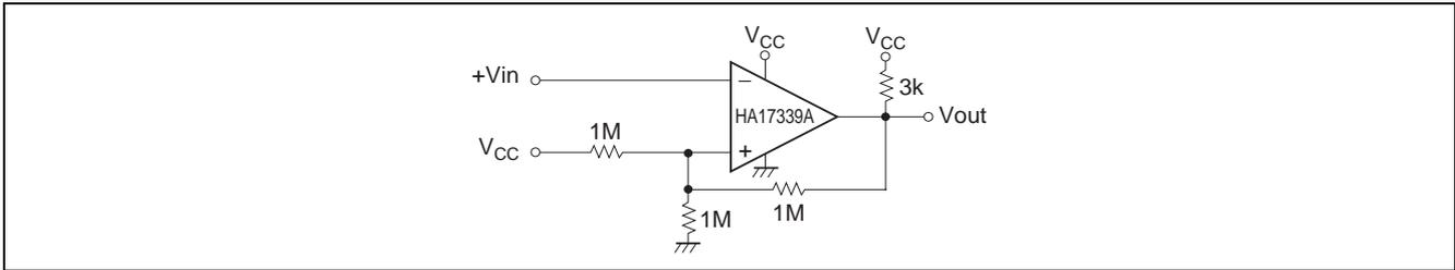
Figure 9 Inverting Comparator
