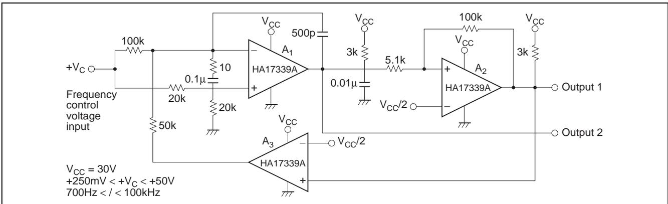
Figure 5 Voltage Controlled Oscillator
