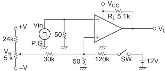
$t_R$ :  $R_L = 5.1k\Omega$ , a 100mV input step voltage that has a 5mV overdrive
