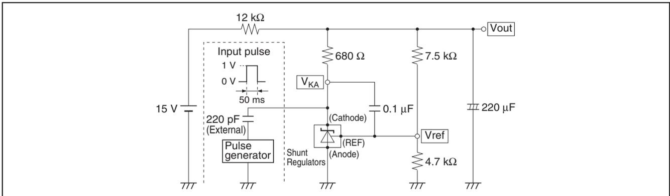
Figure 1 Noise Response Characteristics Measurement Circuit
