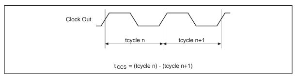
Fig.1 Cycle to Cycle Jitter (3.3V Single Ended Clock Output)
