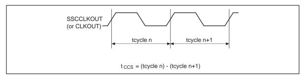
Figure 1 Cycle to cycle jitter
