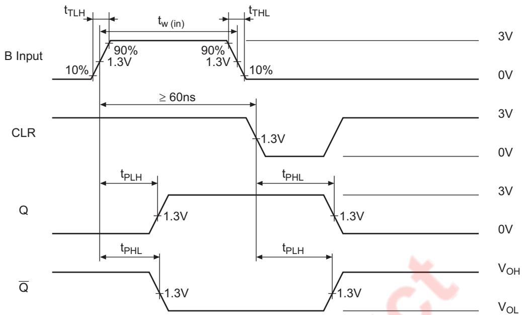
Note: Input pulse:  $t_{TLH} \leq 15 ns$ ,  $t_{THL} \leq 6 ns$ , PRR = 1 MHz
