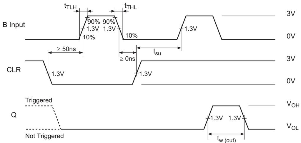
Note: Input pulse:  $t_{TLH} \leq 15\text{ ns}$ ,  $t_{THL} \leq 6\text{ ns}$ , PRR = 1 MHz
