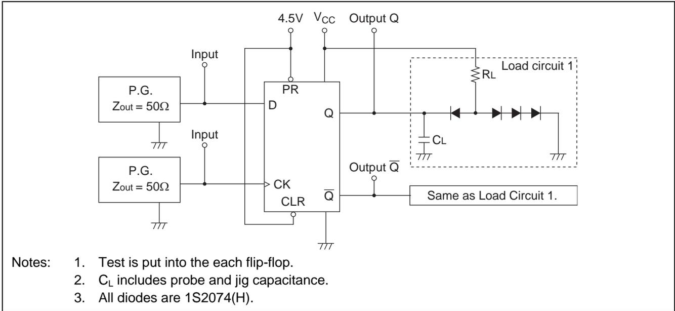
2.  $t_{PHL}$ ,  $t_{PLH}$  (Clear or Preset  $\rightarrow$  Q,  $\bar{Q}$ )
