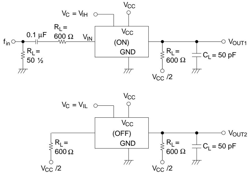
Crosstalk (Control input to signal output)
