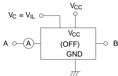
CONDITION 1: V<sub>A</sub> = 0, V<sub>B</sub> = V<sub>CC</sub>
