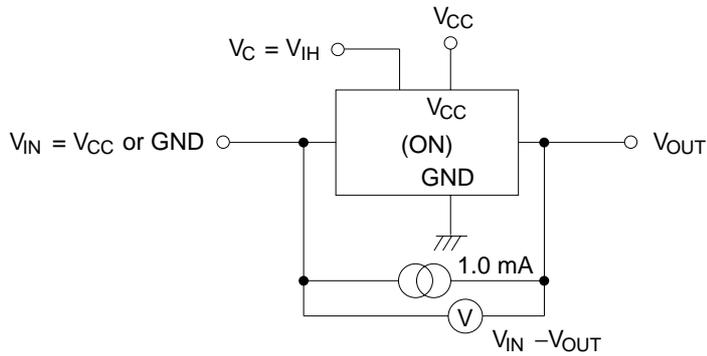
$$R_{ON} = \frac{V_{IN} - V_{OUT}}{10^{-3}} (\Omega)$$
